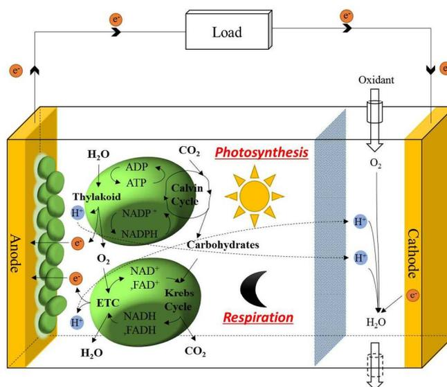
Figure 1. Principle of operation in a bio-solar cell. Schematic representation of the photosynthetic and respiratory electron transport pathways of cyanobacteria.
