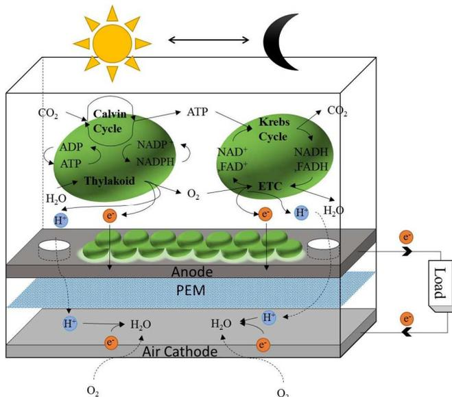
Figure 4. Principles of operation of our new bio-solar cell. The anode structure is designed to face the sun while producing protons that travel toward the cathode through holes at the periphery of the anode.
