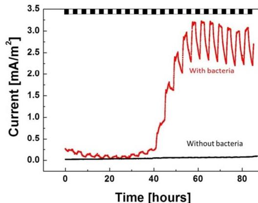
Figure 5. Positive light response of the bio-solar cell under 100 k $\Omega$  resistor. The device was examined under 2 hour light/dark intervals. The white bars indicate the illuminated period and the shadow indicates the dark period.
