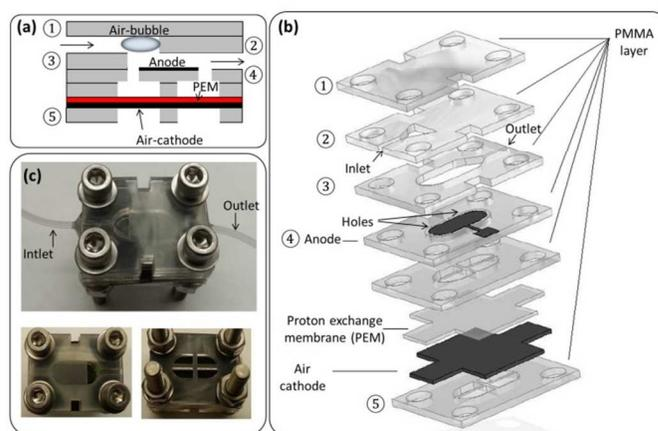
Figure 3. (a) Schematic of the micro-sized bio-solar cell (side view), (b) schematic of the individual layers in the device. There are holes at the periphery of the anode layer. (c) A photo-image of the fully assembled MEMS bio-solar cell, its top-view, and its bottom-view. The cell has a ~300- $\mu\text{L}$  single chamber defined by PMMA and rubber layers.
