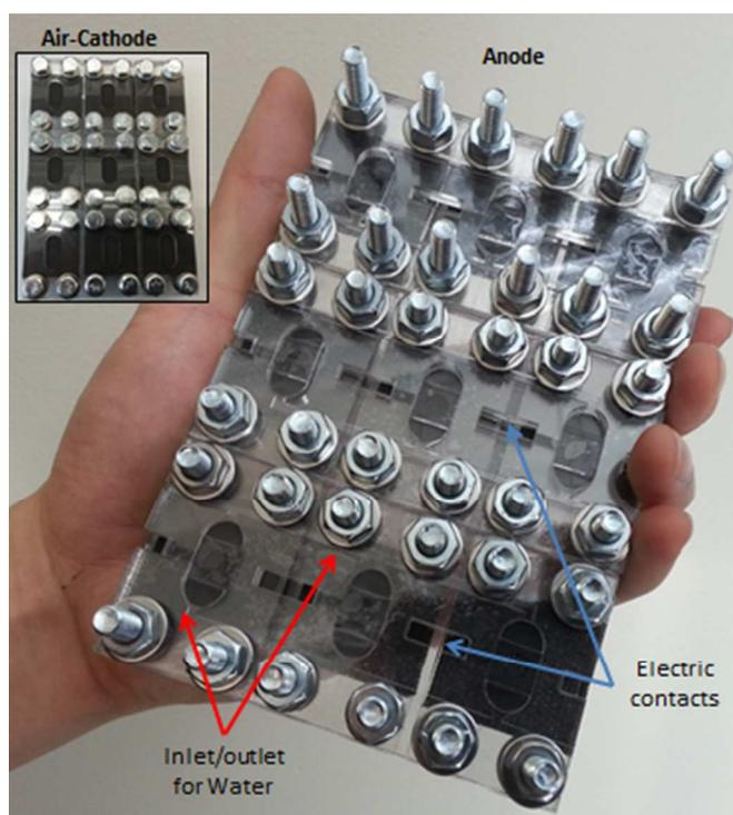
Figure 8. Conceptual 3x3 bio-solar cell array
