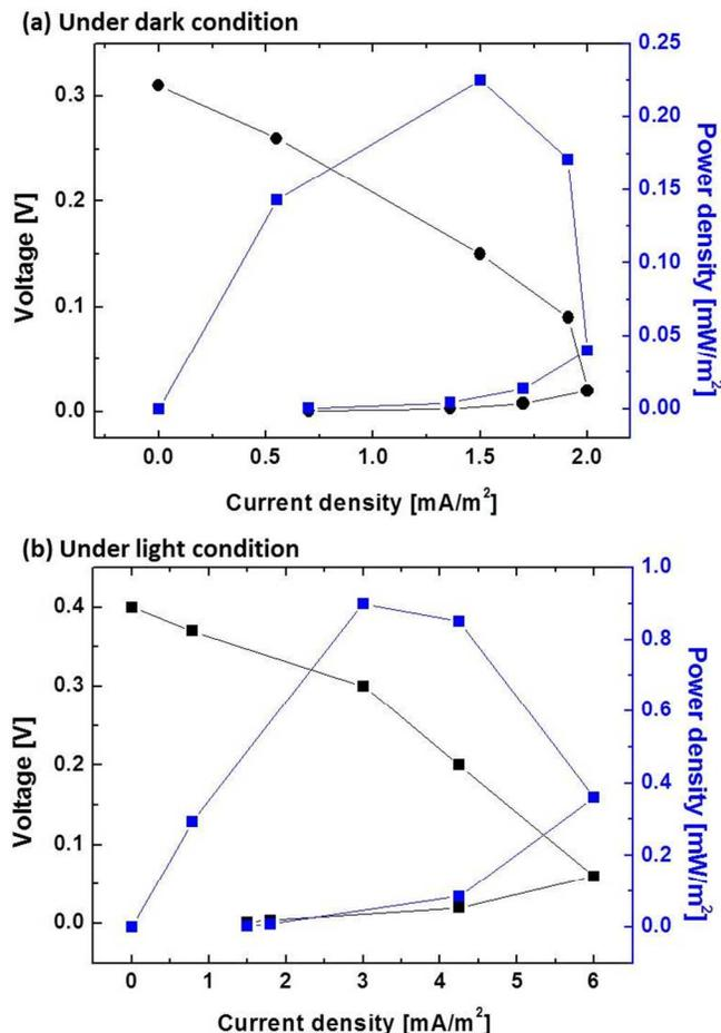
Figure 6. Polarization curve and output power measured as a function of current (a) under dark and (b) light conditions
