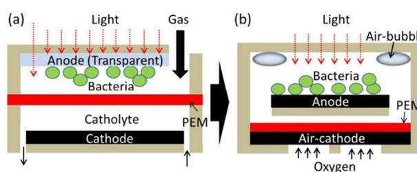
Figure 2. (a) Conventional two-chambered bio-solar cell with face-to-face electrode configuration and open-air system and (b) an innovative single-chambered device proposed in this work with face-up configuration and air-bubble trap
