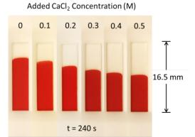
Fig. 3 Photographs of LFA devices showing the transport of citrated whole blood during 240 s for several concentrations of added  $CaCl_2$  solutions.
