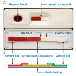
**Fig. 2** Blood coagulation screening using lateral flow in paper-based devices: (a) photographs of an as-used assembled device (top) and of the device with the top piece removed to show the flow and device components; (b) schematic of the flow components.
