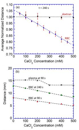
**Fig. 6** Travel distance in LFA as a function of  $CaCl_2$  concentration: (a) normalized distance at 240 s for RBCs in whole blood samples and for dextran solutions; (b) travel of RBCs at 90 s and 240 s and of plasma (in whole blood) samples at 90 s.
