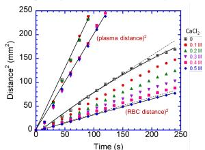
Fig. 4 Transport of RBCs and plasma in LFA devices: (travel distance)<sup>2</sup> vs. time for RBCs and plasma components of whole blood samples.
