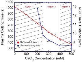
Fig. 8 Comparison between data obtained from RBC travel distance (for 240 s) in LFA device and plasma clotting times obtained with CoaData 2000 Fibrintimer® as a function of  $CaCl_2$  concentration.
