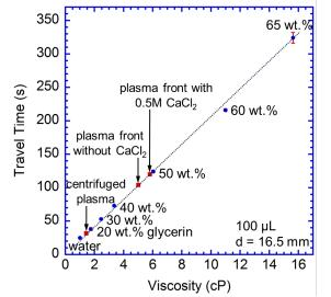
Fig. 5 LFA travel time of glycerin/water samples (blue circles) with similar surface tension vs. their viscosity. Travel time of several plasma samples (red squares) indicate their effective viscosity. Nitrocellulose strip length -16.5 mm.
