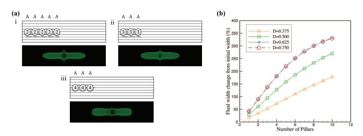
**Fig. 5** (a) Multiple routes to similar *stretch* transformations. Note that three pillars of D/w = 0.625 achieves roughly the same output as five pillars of D/w = 0.5. Moving to a D/w = 0.75 begins the *split* transformation sooner, in addition to flattened ends. (b) (Please view in color) The effect of changing diameter and increasing numbers of central pillars on the stretched width of the central fluid element. Note that D/w = 0.75 and D = 0.625 are functionally identical for this effect.
