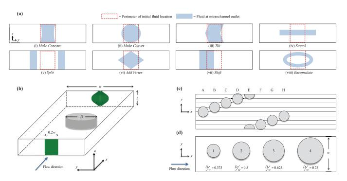
**Fig. 1** (a) Objective transformations. (b) Schematic of microchannel, showing a cross-section of the fluid elements at the inlet (middle 20% being tracked), and a sample deformation induced by a single pillar at the center of the channel. (c) Discretized simulation scheme lettered indices for locations space  $\frac{1}{8w}$  (A-H), and (d) pillar diameters shown with indices 1-4, labelled with true pillar diameter and drawn to scale.
