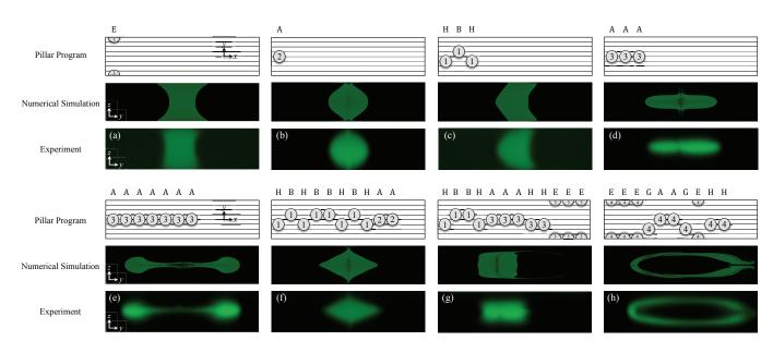
**Fig. 2** Fundamental transformations '*Make Concave*' (a), '*Make Convex*' (b), '*Tilt*' (c), '*Stretch*' (d), and Hierarchical transformations '*Split*' (e), '*Add Vertex*' (f), '*Shift*' (g) and '*Encapsulate*' (h). The figures show the pillar sequence schematic on top, the numerical prediction as an output from uFlow in the middle, and the experimental validation on the bottom.
