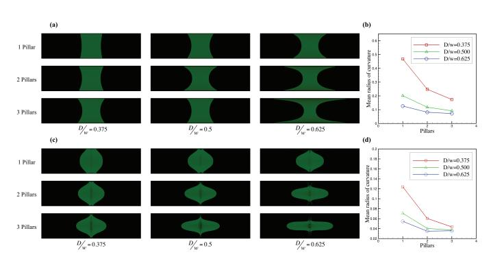
**Fig. 4** Illustrations of (a) *make concave* and (c) *make convex* per pillar type through 3 pillars, and changes in mean radius of curvature vs. number of similar pillars in sequence for (b) the *make concave* and (d) *make convex* operations.
