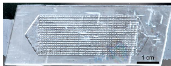
Fig. 5 Microfluidic network (micromodel) etched into a calcite crystal. The trigonal-rhombohedral structure of calcite is apparent as well as inherent natural fractures parallel to the crystal planes
