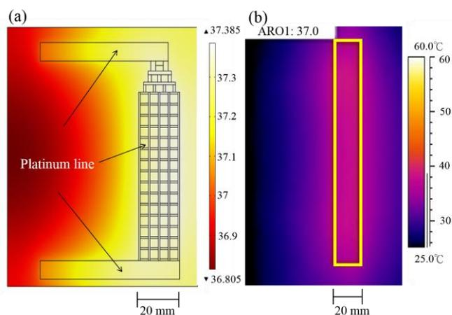
Figure 3. Temperature distribution of a Pt micro-heater generated by (a) simulation and (b) detected with an IR imager. The area marked by the yellow box represents the region of cell-culture maintained at average temperature 37 °C during the experiment.
