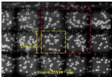
Figure 5. The image in the yellow region shows that CL1-0 cells were seeded in the culture micro-channel, above the micro-heater of grid form; the dimensions of the grid were  $250 \mu\text{m} \times 250 \mu\text{m}$ .
