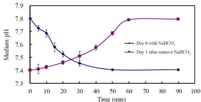
Figure 4. Temporal variation of medium pH in the culture area. When NaHCO<sub>3</sub> (0.8 M) flowed into the CO<sub>2</sub> chamber, the pH of the medium altered from 7.7 to 7.4 (blue line). After cells were cultured one day, we removed NaHCO<sub>3</sub> from the gas chamber. The pH of the medium spontaneously increased from 7.4 to 7.8 in 60 min (purple line). The pH in the culture area was measured with pH test paper.
