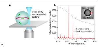
Fig. 4 Lasing of fluorescent E. coli bacterial cells in surface-supported microdroplets.
