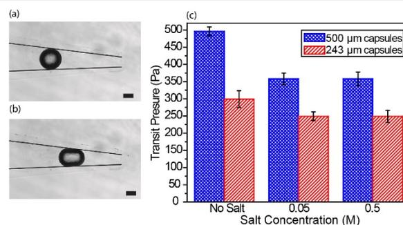
**Figure 4.** Optical image of pressure driven flow of a microcapsule through a tapered capillary: the microcapsule deforms as the pressure is increased from (a) 187 Pa to (b) 249 Pa. The scale bar is 100 μm. Black lines are added to outline the inner boundary of the capillary. (c) Transit pressure for chitosan/*s*-SEBS microcapsules prepared using 0.1 wt.% polymer concentrations and different concentrations of NaCl in the aqueous phase as indicated.
