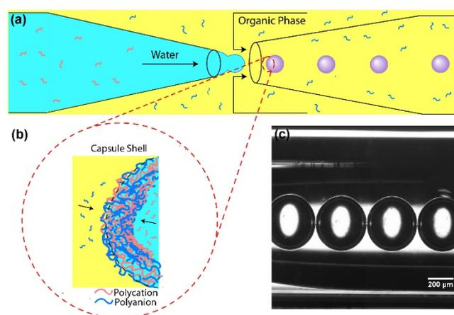
**Figure 1.** Schematic of the capsule fabrication method in a microfluidic device (a) Aqueous phase (turquoise) containing a water soluble polyelectrolyte and an oil phase (yellow) containing oil soluble polyelectrolyte are brought into contact to fabricate aqueous-core microcapsules with a polymeric shell. (b) Electrostatic interaction of the polycation (red) and polyanion (blue) across the droplet interface generates a robust shell with thickness in the range of 1-2  $\mu\text{m}$  (c)
