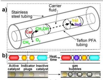
Figure 7. (a) Schematic of a section of Teflon tubing containing droplets inside stainless steel tubing. (b) Schematics (above) and microphotographs (below) show two indicator separating adjacent catalyst plugs to enable clear identification of active catalysts.<sup>41</sup>
