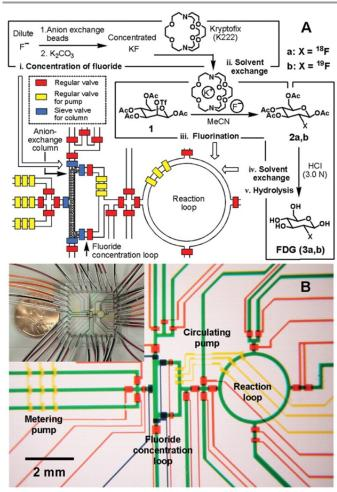
Figure 4. Example of integrated chemical synthesis on chip for the production of 2-deoxy-2-fluoro-d-glucose. The various channels have been loaded with food dyes to help visualize the different components of the microfluidic chip. Reprinted with permission from AAAS.<sup>23</sup>
