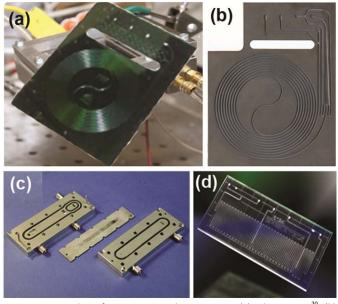
Figure 3. Examples of microstructured reactors in (a) silicon-Pyrex,  $^{20}$  (b) ceramics,  $^{21}$  (c) stainless steel (IMM),  $^{16}$  and (d) glass (Chemtrix).  $^{22}$
