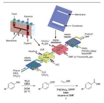
Figure 6. Multistep reaction sequence with liquid-liquid extraction and single stage distillation for solvent switch. $^{30}$
