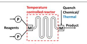
Figure 1. Elements of a continuous flow system. P: Pump; M: Mixer
