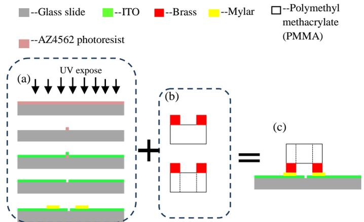
**Fig. 3:** Fabrication process of biochip. (a) ITO-patterned glass slide through standard lift-off process <sup>[51]</sup> and an insulator layer made of 25 mm×25 mm×12  $\mu\text{m}$  in width, length and thick, mylar film. (b) Micro-milled brass fixed on top of polymethyl methacrylate (PMMA) with PMMA adhesive as vertical electrodes and through-hole in the PMMA. (c) Assembly. **Figure not to scale.**
