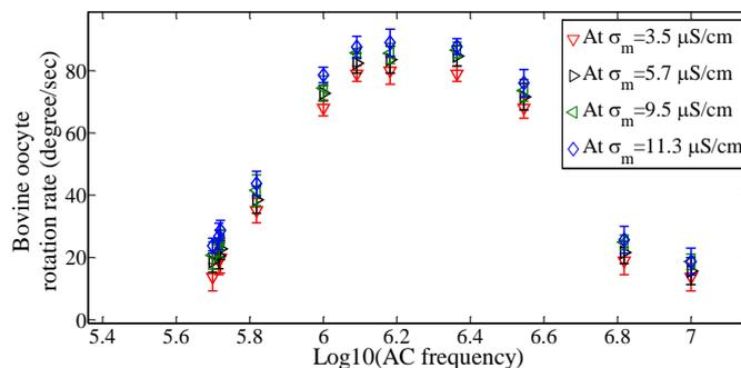
**Fig. 7:** ZP-free bovine oocyte in-plane rotation rate in relation to the conductivity ( $\sigma_m$ ) of buffer medium and the applied frequency in experiment. Here the ac potential amplitude is fixed at 10 V. Based on  $N=4$ ,  $n=3$ . For each frequency, 12 data points from media in different conductivity were analysed by the 2-tailed t-test with equal variance.
