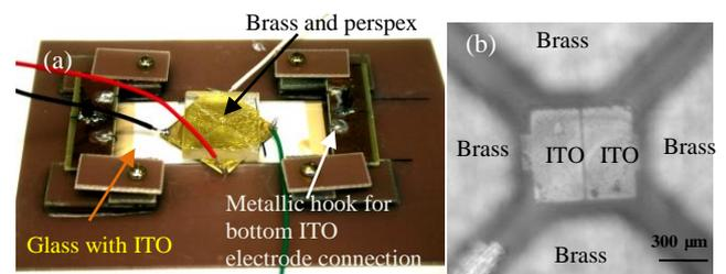
**Fig. 4:** Fabricated biochip. (a) Fabricated biochip with electrical connections. (b) Close-up top view shows sidewall brass and bottom ITO electrodes. The chamber workspace is a 750- $\mu\text{m}$  square area <sup>[48]</sup>.
