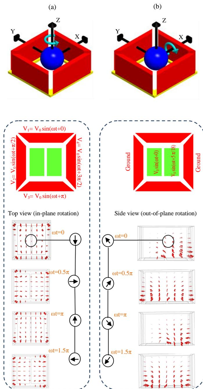
**Fig. 2:** Electric field analysis. (a) In-plane (yaw) rotation: top view. (b) Out-of-plane (pitch) rotation: side view. The first row shows 3D illustration of the rotation about two axes. Complete rotation of electric field for a single period of  $\omega t = 0$  to  $1.5\pi$ , using COMSOL v4.3 FEA software.  $\omega$ -angular frequency of the applied ac electric field and  $t$ -time in seconds. Arrow vectors length and thickness correspond to field strength.
