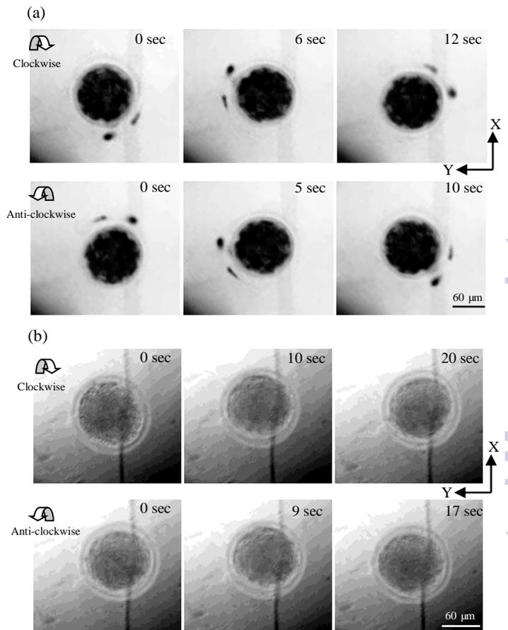
**Fig. 5:** Snapshot of individual bovine oocyte yaw rotation in experiment. Arrows show the rotation direction. Settings for (a) ZP-free oocyte rotation and (b) ZP-intact oocyte rotation, at 10 V, 500 kHz frequency and 90° phase shift between two pairs of orthogonally arranged vertical electrodes.
