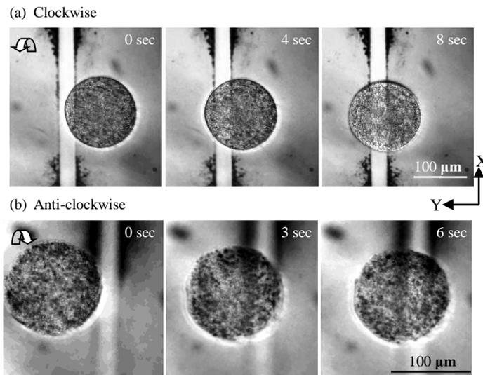
**Fig. 8:** Snapshot of individual bovine oocyte rolling rotation in experiment. (a) Clockwise rotation. (b). Anti-clockwise rotation with larger view of the oocyte (note: lysed oocyte). Settings are 10 V, 40 kHz and 50° phase shift between the two bottom electrodes.
