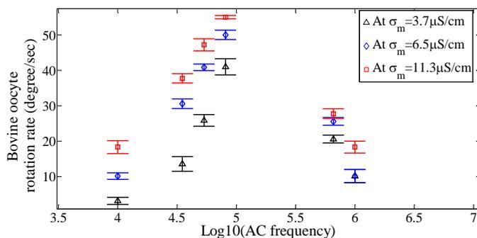
**Fig. 9:** ZP-free bovine oocyte rolling rotation rate in relation to the conductivity of buffer medium and the applied frequency in experiment. Here the potential amplitude is fixed at 10 V. Based on  $N=4$ ,  $n=3$ .
