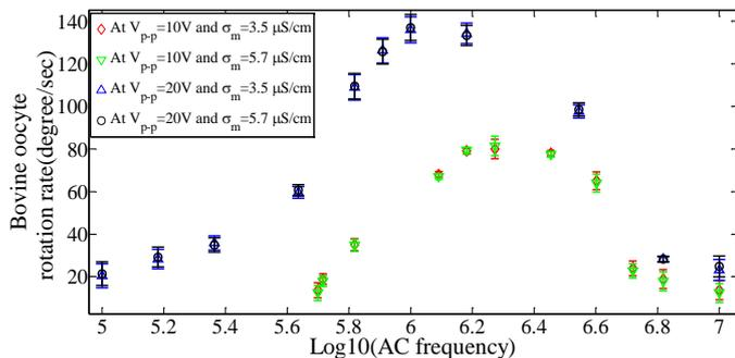
**Fig. 6:** ZP-free bovine oocyte in-plane rotation rate in relation to the conductivity ( $\sigma_m$ ) of buffer medium and the applied ac potential (frequency and amplitude  $V_{p-p}$ ) in experiment. Based on 4 oocytes  $\times$  3 replicates ( $N=4$ ,  $n=3$ ) with  $N$  being the number of samples and  $n$  being the number of technical replicates.
