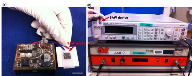
**Fig. 1** (a) Initial prototype of the battery-powered circuit to be used to drive the SAW microfluidic aerosol delivery platform (scale bar = 1 cm). (b) Typical signal generator and amplifier used in laboratory settings to provide sufficient power for SAW nebulization (scale bar = 3 cm).
