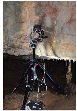
Fig3: Portable XRF apparatus implemented in La Garma cave.
