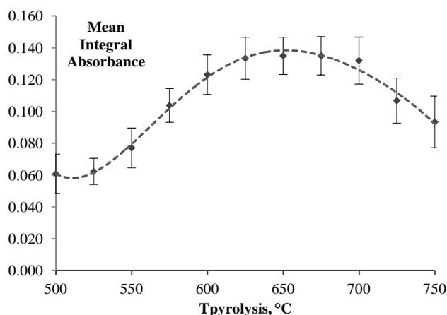
Fig. 2 Dependence of As absorbance on arsine pyrolysis temperature, error bars denote  $\pm$ SD (1000 pg As,  $n = 5$ )
