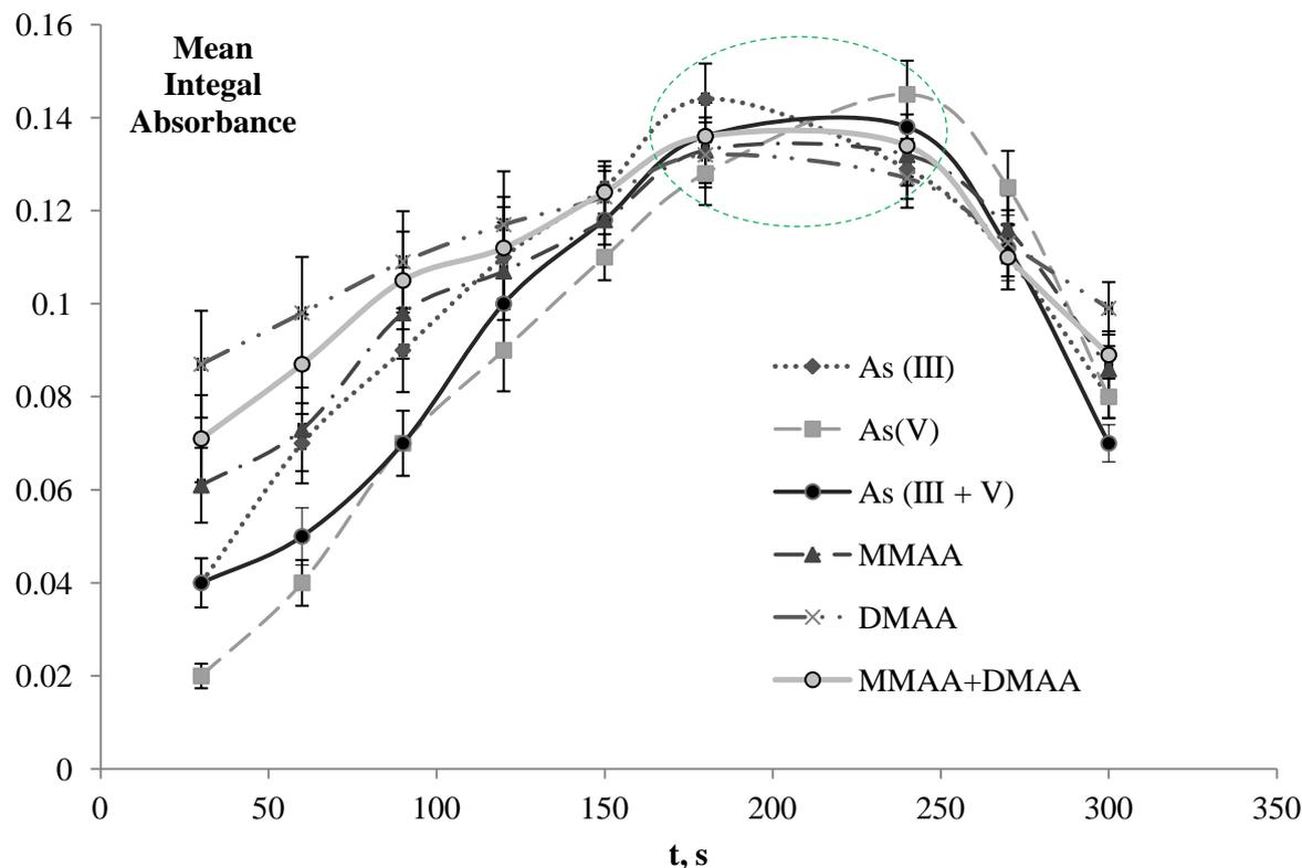
**Fig. 5** Time dependence of arsenic absorbance for solutions containing As(III) 10  $\mu\text{g/L}$ ; As(V) 10  $\mu\text{g/L}$ ; As(III) 5  $\mu\text{g/L}$  + As(V) 5  $\mu\text{g/L}$ ; MMAA 10  $\mu\text{g/L}$ ; DMAA 10  $\mu\text{g/L}$ ; MMAA 5  $\mu\text{g/L}$  + DMAA 5  $\mu\text{g/L}$  ( $n = 5$ ). Dashed green circle marks the area where all studied arsenic species contributes equally to the analytical signal, error bars denote  $\pm\text{SD}$
