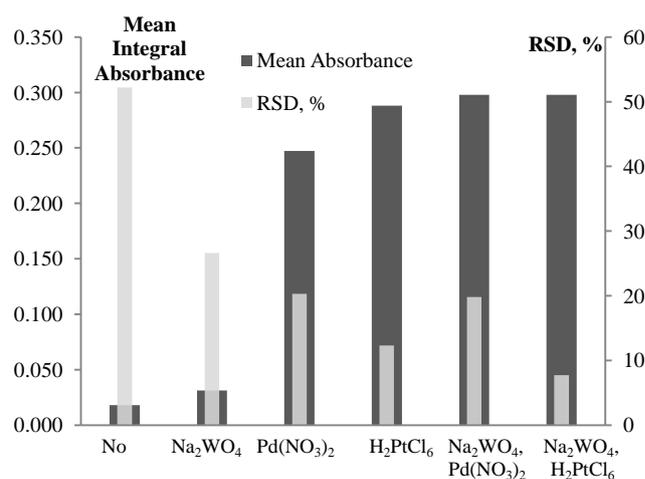
Fig.1 Optimization of graphite furnace coating (2000 pg As, n = 5)
