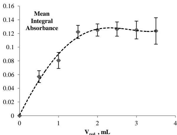
Fig. 3 Dependence of As absorbance on reductant solution quantity, error bars denote  $\pm$ SD (1000 pg As,  $n = 5$ )
