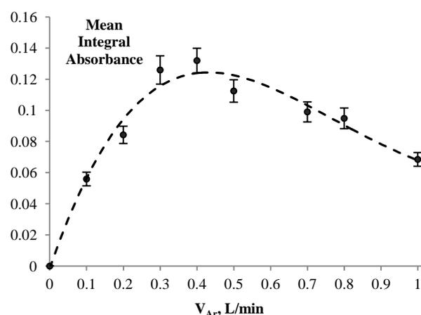
Fig. 4 Dependence of As absorbance on transporting gas flow rate, error bars denote  $\pm$ SD (1000 pg As,  $n = 5$ )
