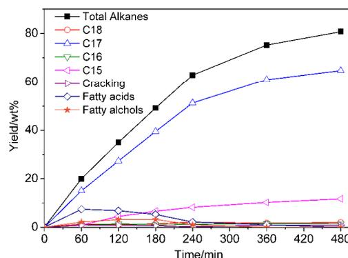
**Fig. 2** Product distribution for the transformation of Jatropa oil over  $\text{Ru}/\text{La}(\text{OH})_3$  at 200 °C as a function of time. Reaction conditions: 0.2 g Jatropa oil, 0.2 g  $\text{Ru}/\text{La}(\text{OH})_3$ , 200 °C, and stirring at 1000 rpm.
