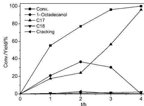
**Fig. 4** The conversion of stearic acid. Reaction conditions: 1 mmol *n*-octadecanol, 0.2 g Ru/La(OH)<sub>3</sub>, 200 °C, 4 MPa H<sub>2</sub>, and stirring at 1000 rpm.
