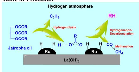
Ruthenium supported on  $\text{La}(\text{OH})_3$  display good performance on the hydrodeoxygenation of fatty acid and Jatropha oil at 200 °C.
