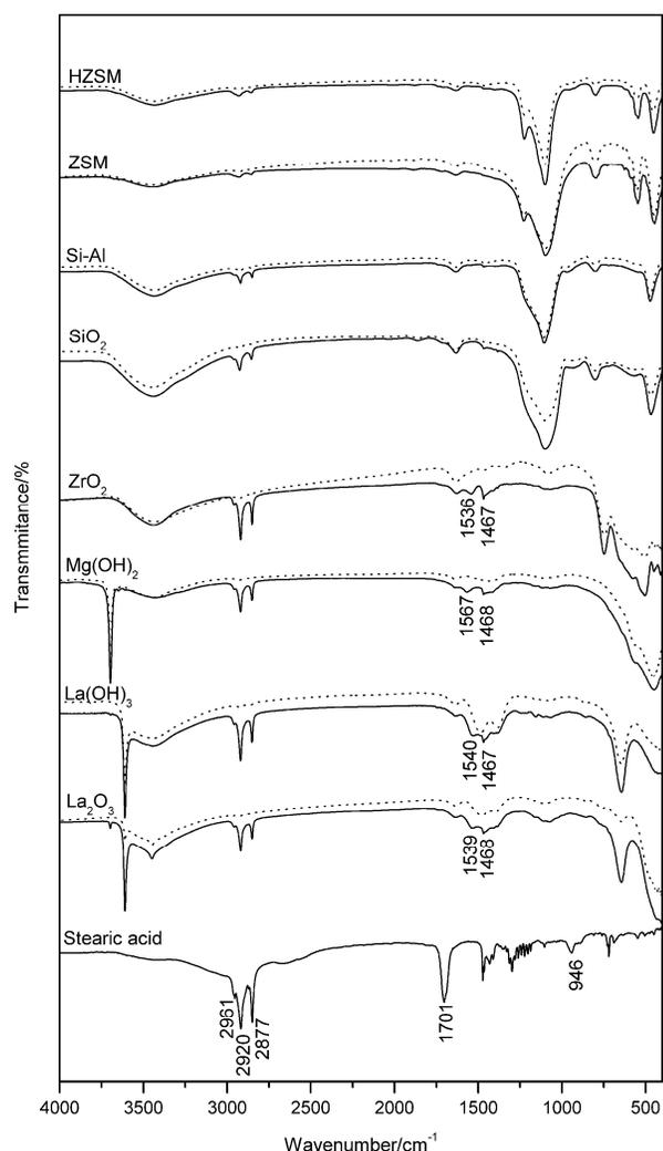
**Fig. 1** IR spectrums of the supports. The dot lines represent the untreated supports, and the solid lines represent the treated supports.
