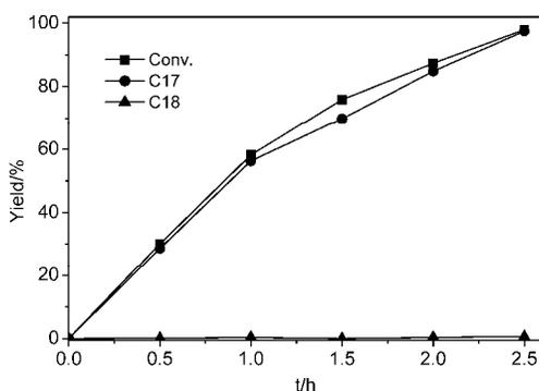
**Fig. 5** The conversion of *n*-octadecanol. Reaction conditions: 1 mmol *n*-octadecanol, 0.2 g Ru/La(OH)<sub>3</sub>, 200 °C, 4 MPa H<sub>2</sub>, and stirring at 1000 rpm.
