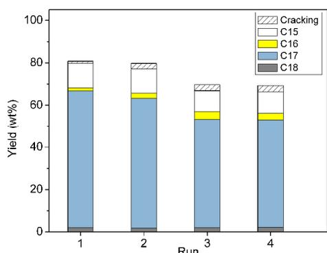
**Fig. 3** The performance of the catalyst in the recycle experiment.
