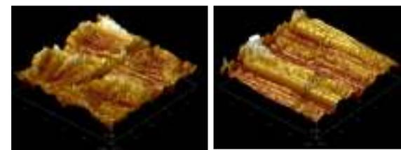
**Figure 4.** Topographic imaging of the original stainless steel (left) and the modified SS-QAS, **3** (right) performed in the tapping mode with a scan rate of 1.0 Hz at fixed resolution (512  $\times$  512 data points).
