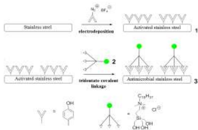
**Figure 2.** Grafting antibacterial QAS to a stainless steel surface.
