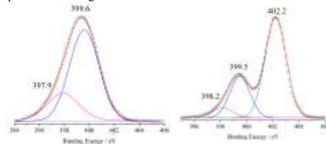
**Figure 3.** Al K $\alpha$  excited XPS of left) SS-phenol, **1**; right) SS-QAS, **3** in the N 1s energy region. The black dots represent the experimental profile. The red line superimposed to the experimental profile refers to the sum of the components. Left) The magenta and blue lines refer to the 397.9 and 399.6 eV components, respectively. Right) The magenta, blue and green lines refer to the 398.2, 399.5 and 402.2 eV components, respectively.
