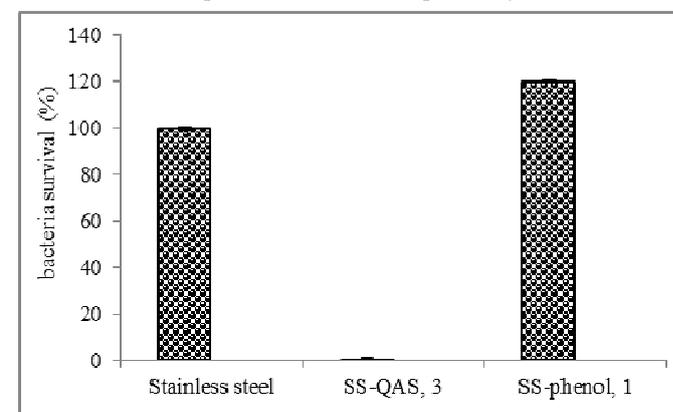
**Figure 5.** Survival of *E. coli* ATCC 25922 after treatment with control and modified materials. The results represent the mean and standard errors (SD) of three independent biological experiments done in triplicates.
