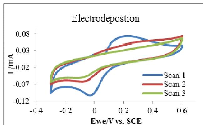
**Figure 1.** Electrodeposition of diazonium salt. Scan rate 0.25mV/s.
