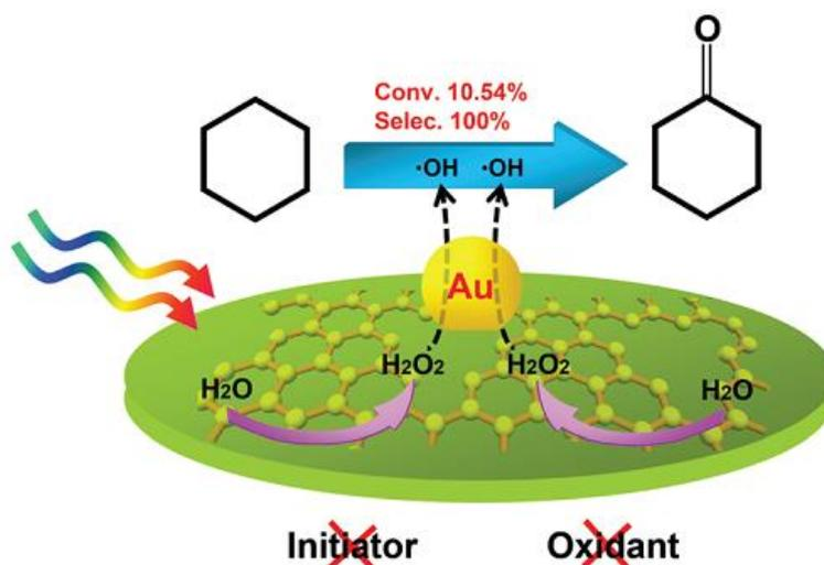
**Scheme 10.** Proposed reaction mechanism for visible-light driven oxidation of cyclohexane on  $C_3N_4$ /Au,<sup>108</sup> reproduced by permission of The Royal Society of Chemistry.
