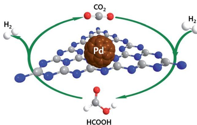
**Scheme 19.** Pd/mpg-C<sub>3</sub>N<sub>4</sub> catalyzed hydrogen production and storage,<sup>172</sup> reproduced by permission of The Royal Society of Chemistry.
