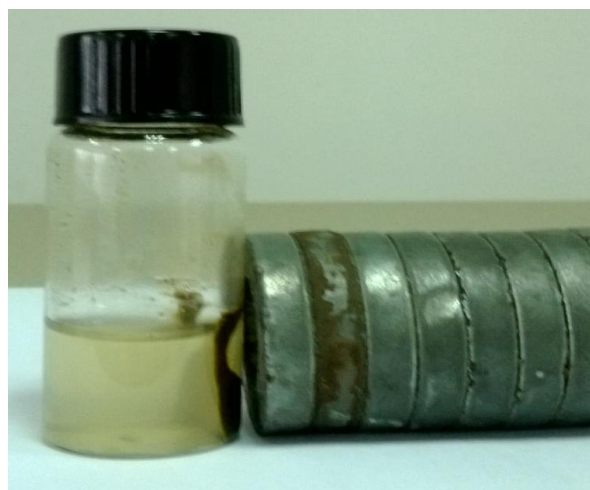
Fig. 8 Recycle of the catalyst by an external magnet.
