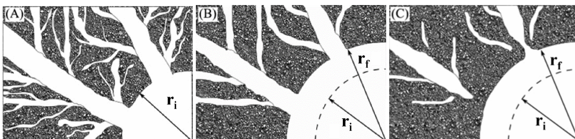
Fig. 4. Schematic graphical representation of the dissolution of silica from regions of small positive radius of curvature at the intersection of the secondary pore network and the primary mesopores of radius r_i , and redeposition in micropores as well as the entrance to the secondary pore network in regions of small negative radius of curvature. In the process (top to bottom), the void fraction decreases and the mesopore diameter increases from r_i to r_f . 41 Reprinted with permission from Ref. 41 (Rachel A. Pollock, Gennady Yu. Gor, Brenna R. Walsh, Jason Fry, I. Tyrone Ghampson, Yuri B. Melnichenko, Helmut Kaiser, William J. DeSisto, M. Clayton Wheeler, and Brian G. Frederick, J. Phys. Chem. C 2012, 116, 22802-22814). Copyright (2014) American Chemical Society.
