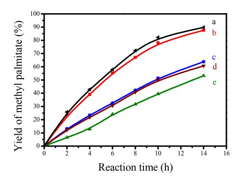
**Figure 5** Dependences of catalytic activities on the time in transesterification of tripalmitin with methanol catalyzed by (a)  $[C_3vim][SO_3CF_3]$  (the same number of acidic sites as that of GNC- $[C_3N][SO_3CF_3]$ ), (b) GNC- $[C_3N][SO_3CF_3]$ , (c)  $H_3PW_{12}O_{40}$ , (d) SBA-15-SO<sub>3</sub>H and (e) Amberlyst 15.
