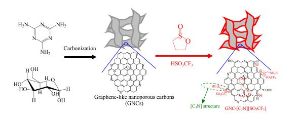
Scheme 1 The procedures for synthesizing GNC-[C<sub>3</sub>N][SO<sub>3</sub>CF<sub>3</sub>].
