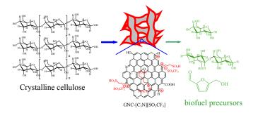
Strong acid ionic liquids and sulfonic groups bifunctional graphene-like nanoporous carbon with abundant nanopores, controlled acidity and excellent catalytic activity for biomass transformation have been successfully prepared in this work.
