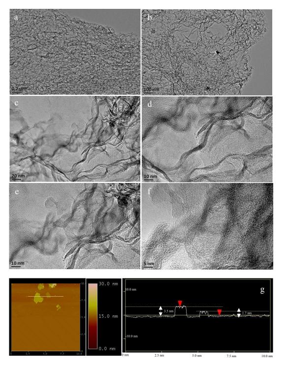
**Figure 2** (a, b) TEM images, (c-f) high-resolved TEM images, and (g) AFM image and corresponding thickness analysis of GNC-[C<sub>3</sub>N][SO<sub>3</sub>CF<sub>3</sub>].
