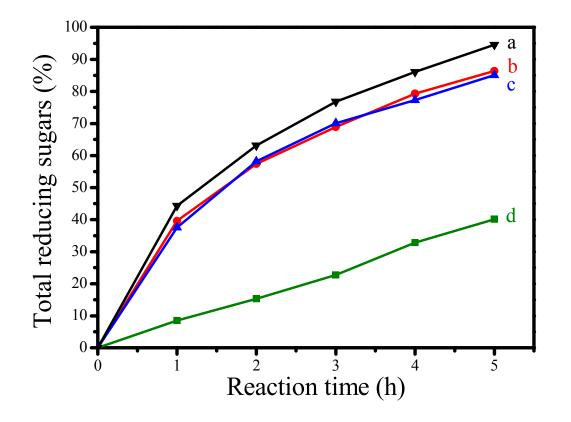
**Figure 6** Dependences of catalytic activities on the time in depolymerization of Avicel into sugars catalyzed by (a)  $GNC-[C_3N][SO_3CF_3]$ , (b) HCl, (c)  $[C_3vim][SO_3CF_3]$  and (d) Amberlyst 15 (b, c, d was used the same number of acidic sites as in  $GNC-[C_3N][SO_3CF_3]$ ).
