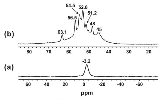
**Figure 4** Room temperature <sup>31</sup>P MAS NMR spectra of adsorbed (a) TMP acquired with proton decoupling, and (b) TMPO of GNC-[C<sub>3</sub>N][SO<sub>3</sub>CF<sub>3</sub>].
