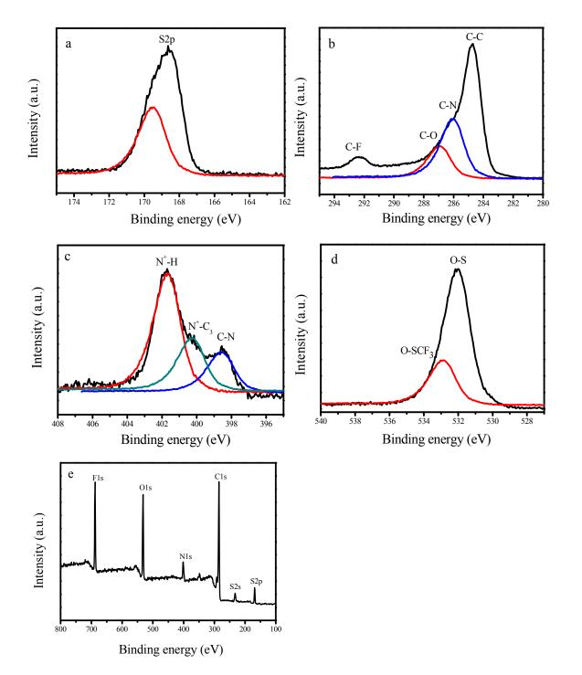
Figure 3 XPS spectra of (a)  $S_{2p}$ , (b)  $C_{1s}$ , (c)  $N_{1s}$ , (d)  $O_{1s}$  and (e) survey of GNC-[C<sub>3</sub>N][SO<sub>3</sub>CF<sub>3</sub>].
