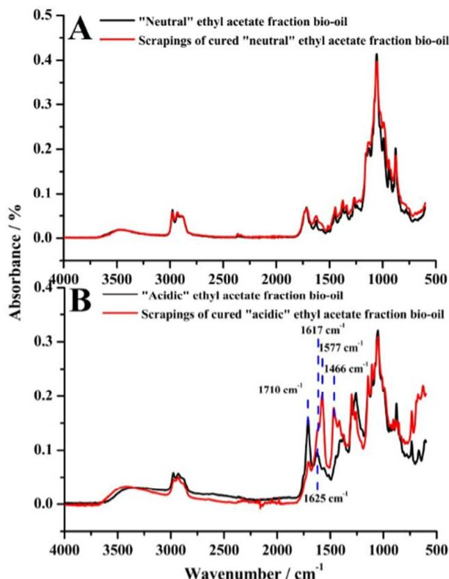
**Fig. 13** ATR-IR spectra of (A) "neutral" ethyl acetate fraction bio-oil and scrapings of cured polymer of this fraction (B) "acidic" ethyl acetate fraction bio-oil and scrapings of cured polymer of this fraction (cured at 160 °C for 4 h).
