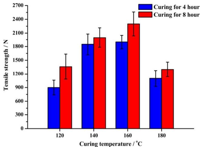
**Fig. 9** Tensile strengths of organic phase bio-oil cured shot-blasted Al plates.
