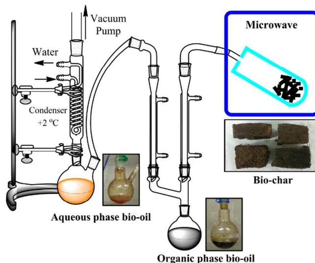
**Fig. 1** Experimental set-up for microwave-assisted pyrolysis of milled waste office paper.
