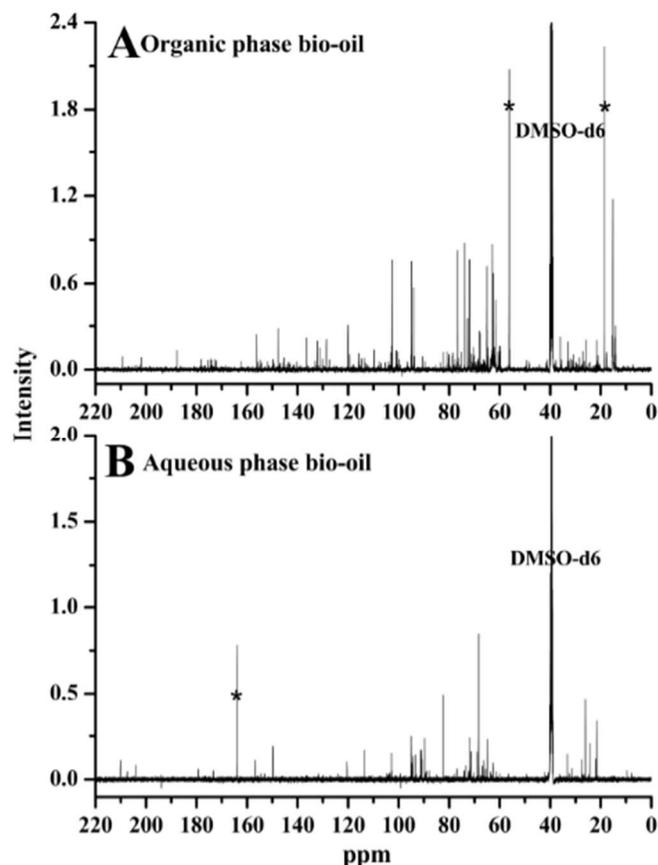
**Fig. 4**  $^{13}\text{C}$  NMR spectra of (A) organic phase bio-oil, (B) aqueous phase bio-oil. (All spectra used the central resonance of DMSO- $d_6$  ( $\delta\text{C}$ , 39.52 ppm) as the internal reference).
