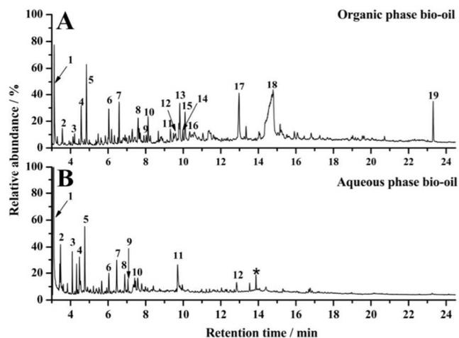
**Fig. 5** GC-MS spectra of (A) organic and (B) aqueous phase bio-oils derived from MW-assisted pyrolysis of milled waste office paper
