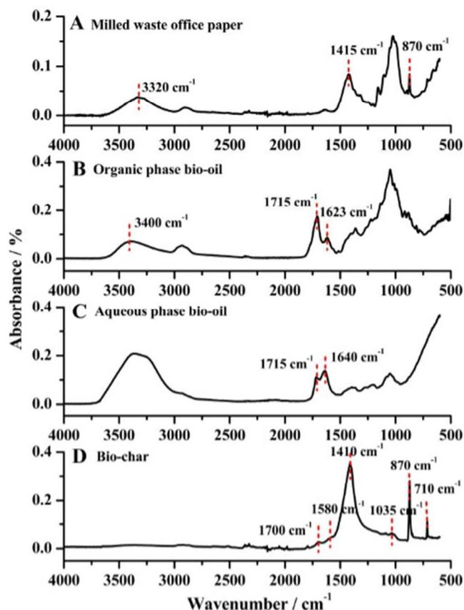
**Fig. 3** ATR-IR spectra of (A) milled waste office paper (B) organic phase bio-oil (C) aqueous phase bio-oil (D) bio-char.
