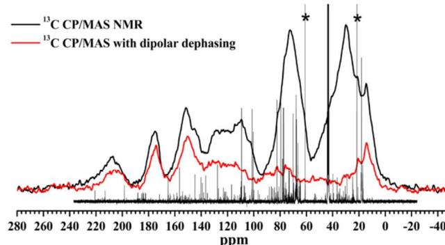
**Fig. 11** Solid-state  $^{13}\text{C}$  CP/MAS NMR spectrum of bio-oil/Al scraping (black) and  $^{13}\text{C}$  CP/MAS NMR spectrum of bio-oil/Al scraping with dipolar dephasing (red), overlapped with liquid-state  $^{13}\text{C}$  NMR of organic phase bio-oil
