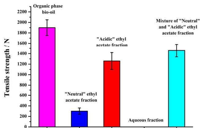
**Fig. 12** Tensile strengths of organic phase bio-oil, "neutral" and "acidic" ethyl acetate and aqueous fraction bio-oil, and mixture of the "neutral" and "acidic" ethyl acetate fraction bio-oil cured Al plates (samples cured at 160 °C for 4 h).
