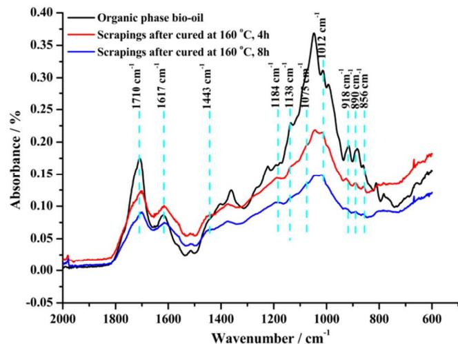
**Fig. 10** ATR-IR spectra of organic phase bio-oil, scrapings of the Al – bio-oil – Al interface polymer formed at 160 °C for 4 and 8 h cure.
