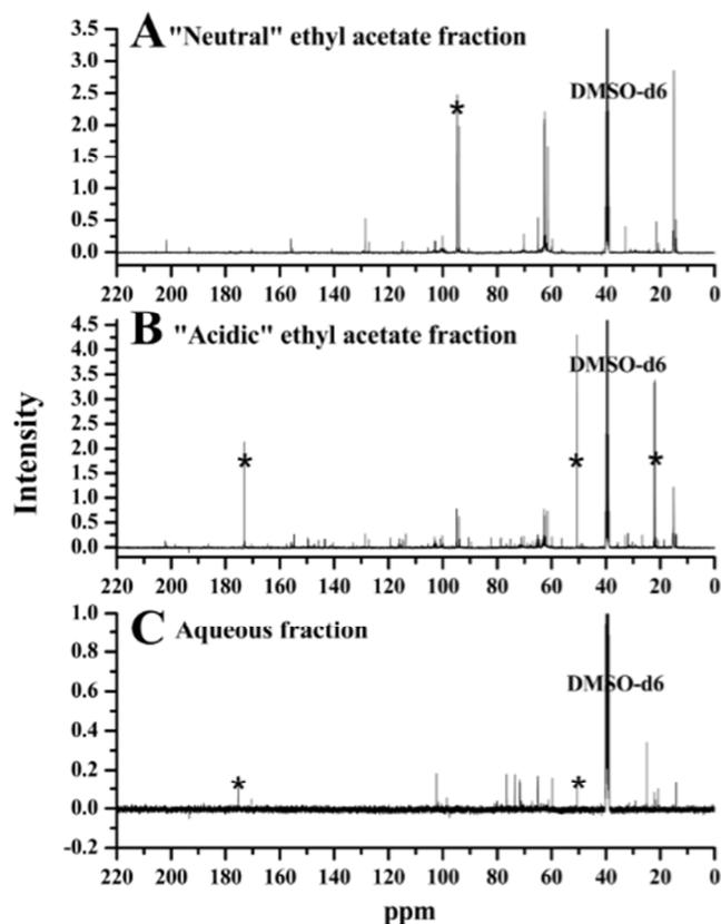
**Fig. 7** <sup>13</sup>C NMR spectra of (A) "Neutral" ethyl acetate fraction (B) "Acidic" ethyl acetate fraction (C) Aqueous fraction bio-oil. (All spectra used the central resonance of DMSO-d<sub>6</sub> ( $\delta$ C, 39.52 ppm) as the internal reference)
