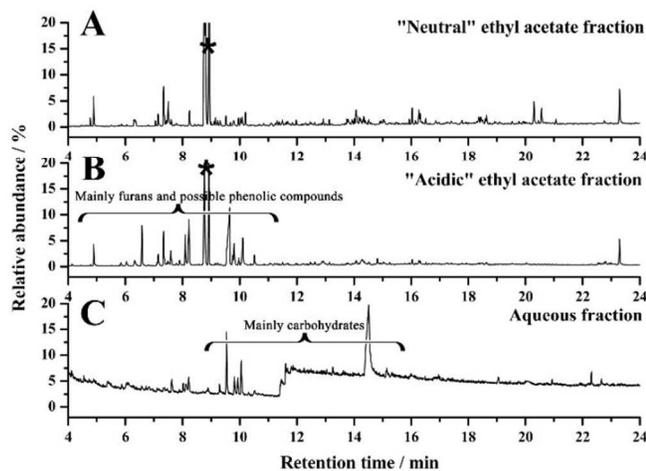
**Fig. 8** GC-MS spectra of (A) “neutral”, (B) “acidic” ethyl acetate fraction and (C) aqueous fraction bio-oil resulted from liquid-liquid separation of organic phase bio-oil
