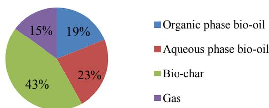
**Fig. 2** Yield of low temperature microwave-assisted pyrolysis products.
