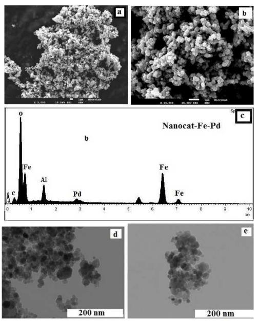
Figure 4. SEM images of Nanocat-Fe-Pd a and b; c) EDS profile of Nanocat-Fe-Pd d) TEM image of Fe<sub>3</sub>O<sub>4</sub> and e) TEM image of Nanocat-Fe-Pd
