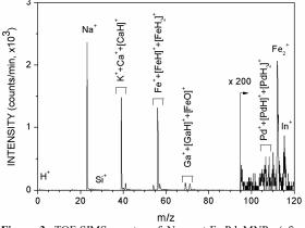
Figure 3. TOF-SIMS spectra of Nanocat-Fe-Pd MNPs (after 30 s of sputtering)
