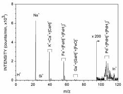
Figure 2. TOF-SIMS spectra of Nanocat-Fe-Pd MNPs (surface)
