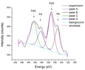
**Figure 1**. XPS spectrum of Pd 3d line. The expected line positions in the 65 case of metallic Pd and PdO are marked by arrows.
