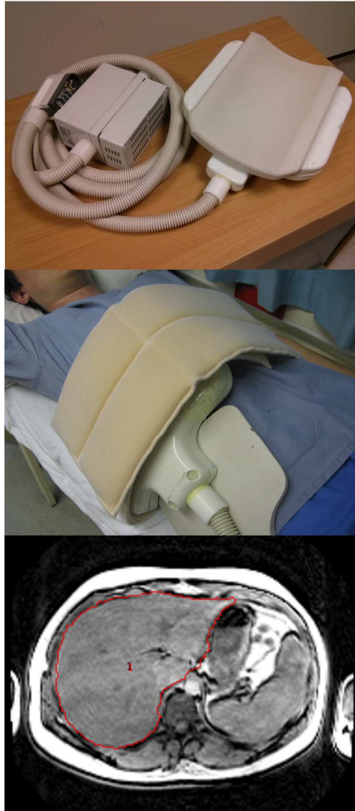
Figure 1. Picture showing Pulseteq ^{13}\text{C} surface coil with quadrature proton decoupling coil used for glycogen signal detection (top), position of subject for scanning routine (middle), and T_1 weighted gradient echo sequence MR image of liver (bottom) showing region of interest (red outline). The gastric content of the stomach is also visible.
