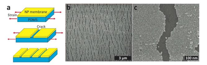
**Figure 2.** (a) Sketch of nanoparticle membranes deposited onto PDMS substrates, showing crack formation under applied tensile strain. (b) SEM image of crack formation in 5.2 nm Audodecenthiol nanoparticle monolayer under the applied strain of 20%. (c) Zoomed in image of a particular crack, making it possible to identify individual nanoparticles. Images (b) and (c) were taken by SEM after the strained monolayer had been transferred from the PDMS to a silicon substrate.
