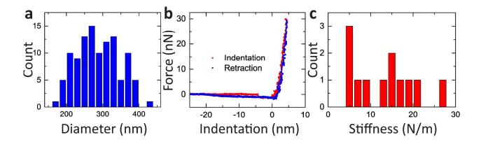
**Figure 7** (a) Histogram of the diameter distribution for nanoparticle scrolls fabricated as shown in Fig. 6. (b) Typical force-indentation curve obtained by AFM. The tip comes is in contact with the scroll for positive indentation values. (c) Histogram of the stiffness values from the central region of different scrolls. All data are from scrolls fabricated with 5.2nm Au-dodecanethiol nanoparticles.
