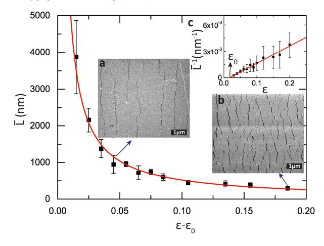
**Figure 3.** Average fragment width  $\overline{L}$  as function of strain  $\varepsilon - \varepsilon_0$  for 5.2 nm Au-dodecanethiol nanoparticle monolayers. Here  $\varepsilon_0$  is the onset strain (see text). The two SEM images show the crack patterns for 6%(a) and 20%(b) strain. Inset c: Determination of the onset strain  $\varepsilon_0$ .
