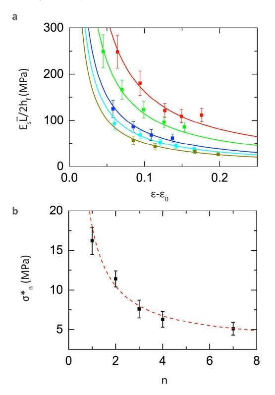
Figure 4. (a) Normalized fragment width as a function of strain beyond onset for multilayers of 9.1 nm Au-dodecanethiol nanoparticles. Solid lines indicating power laws with exponent -1, as in Eq.2. (b) Dependence of the effective fracture strength  $\sigma_n^*$  on film thickness, parameterized by Immediately apparent is that the fracture strength  $\sigma_n^*$  decreases with increasing number of layers
