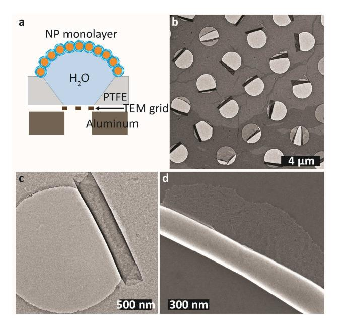
**Figure 6.** (a) Schematic of nanoparticle scroll assembly and transfer process. (b) TEM image of nanoparticle scrolls formed on a carbon-coated TEM grid with 2µm diameter holes via sponateous self-rolling during the drying process. (c) Zoomed in TEM image of a nanoparticle scroll showing individual particles and the wall thickness. (d) SEM image of a nanoparticle scroll transferred onto a silane-coated silicon-nitride substrate.
