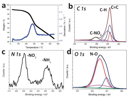
Figure 3. Analysis of *p*-nitrobenzyl functionalized carbon nanofibers. (a) Thermal gravimetric analysis in dry N<sub>2</sub> with heating rate 10 °C / min.; X-ray photoelectron spectra of (b) C 1s; (c) N 1s; (d) O 1s.
