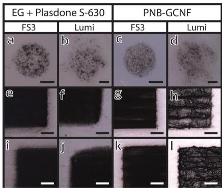
**Figure 4.** Graphene based inks printed on (a, e, i and c, g, k) – FS3 and (b, f, j and d, h, l) - Lumi papers. Expanded graphite with Plasdone S-630 (a and b) – dot, (e, i and 15 f, j) – large-area rectangle, 10 printing passes. *p*-Nitrobenzyl functionalized graphene (c and d) – dot, (g, k and h, l) – large-area rectangle, 10 printing passes. Scale bars: (a-d) – 20  $\mu$ m, (e-l) – 500  $\mu$ m.
