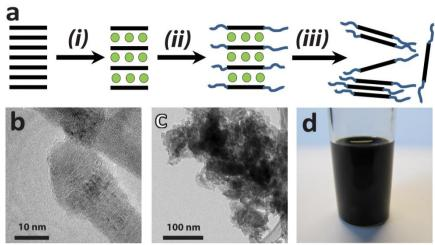
**Figure 2.** Preparation of functionalized graphene inks from graphitic carbon nanofibers (GCNF). (a) Scheme of GCNF functionalization (i) preparation of potassium-GCNF IC, (ii) functionalization of potassium-GCNF IC with *p*-nitrobenzylbromide, and (iii) liquid phase exfoliation; (b) Transmission electron micrograph of starting GCNF; (c) Transmission electron micrograph of cast-dried functionalized GCNF; (d) PNB-GCNF dispersion with concentration of 3 mg/ml in propylene glycol diacetate.
