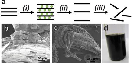
**Figure 1.** Preparation of graphene inks from raw graphite via intercalation. (a) <sup>5</sup> Overall scheme showing: (i) graphite intercalation, (ii) thermal expansion, and (iii) liquid phase exfoliation; (b) Scanning electron micrograph of Li(THF) graphite intercalation compound; (c) Scanning electron micrograph of expanded graphite; (d) Graphene dispersion with concentration of 1.4 mg/ml prepared from expanded graphite.
