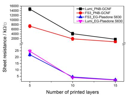
**Figure 5.** Sheet resistance of printed  $5 \times 35$  mm rectangles as a function of number of printing passes.
