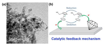
Fig. 1 - (a) TEM micrograph of 10 nm nanodiamond. (b) Illustration of the nanodiamond feedback mechanism. The green arrows depict the direction of electron transfer.
