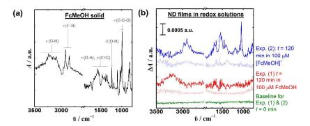
**Fig. 7** – ATR-FTIR spectrum of FcMeOH (solid powder, black line) and (c) ATR-FTIR difference spectra (coloured lines) recorded for solutions of FcMeOH (red) and FcMeOH<sup>+</sup> (blue) on a clean ATR prism (transparent lines) and in the presence of a nanodiamond drop-cast film (solid lines). All 5 aqueous solution contained KCl (0.1 M, pH 5.88).
