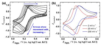
**Fig 6** – (a) Normalised current (by max) voltammograms of FcMeOH (1  $\mu$ M) for scan rates 1, 2, 5 10, 20, 50, 100, 200 and 500 mV s<sup>-1</sup>. (b) Voltammograms of FcMeOH (10  $\mu$ M) for scan rates 2, 20 and 200 mV s<sup>-1</sup>. Experiments were performed with a 300 s pre-experiment equilibration time (no sapplied potential) in KCl electrolyte solution (0.1 M, pH 5.88) on a nanodiamond-modified (5 nm) BDD electrode.
