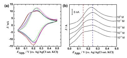
**Fig. 5** – (a) Cyclic Voltammograms ( $5^{th}$  scan) of FcMeOH ( $1\mu$ M) in aqueous solutions containing various concentrations of KCl ( $10^0$ - $10^{-4}$  M, pH = 5.06-6.12 respectively) on a nanodiamond modified (100 nm) BDD working electrode at 5 mV s<sup>-1</sup>. (b) Stacked plot of only the oxidation 5 process. The blue dashed line identifies the standard FcMeOH diffusion controlled peak (as seen for at clean BDD), whereas the red dashed line highlights the emerging pre-peak.
