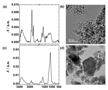
Fig. 2 – ATR-FTIR spectra and TEM micrograph of 5 nm, (a) and (b), and 100 nm, (c) and (d), nanodiamond drop-cast films
