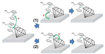
**Fig.8** – Illustration of nanodiamond surface adsorbed FcMeOH<sup>+</sup> and its associated redox reaction. Re-oxidation of the FcMeOH product can then occur by either (1) the underlying electrode (when at sufficient potential) or (2) reaction with nanodiamond surface functionalities. The green arrows 5 depict the direction of electron transfer.
