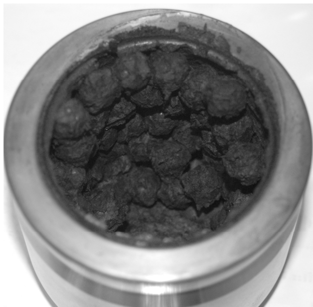
25 Figure 7. Oxidation of graphite in a planetary mill using UHPA results in the formation of a solid mixture that does not tumble.
