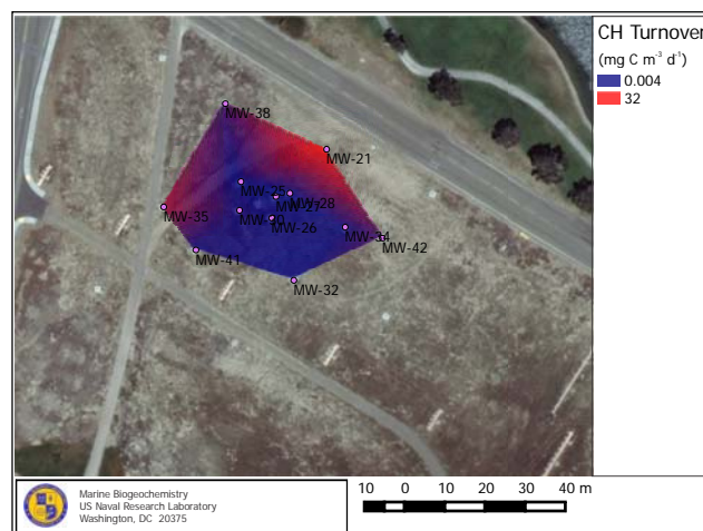
Fig. 4. Contaminant mineralization rate per unit time and area (g C m -3 d -1 ).
