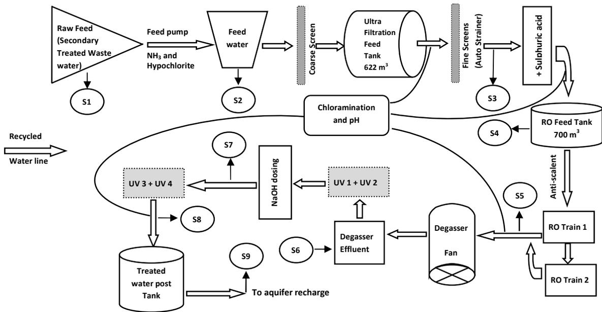
Figure. 1. Schematic of the Beenyup AWRP showing treatment processes and sampling locations.
