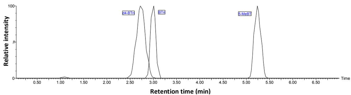
Figure 2. A Combined chromatograms from LC-MS analysis of BTri ( $m/z$  120.055), 5-MeBT ( $m/z$  134.069) and 4d-BTri ( $m/z$  124.083; internal standard).
