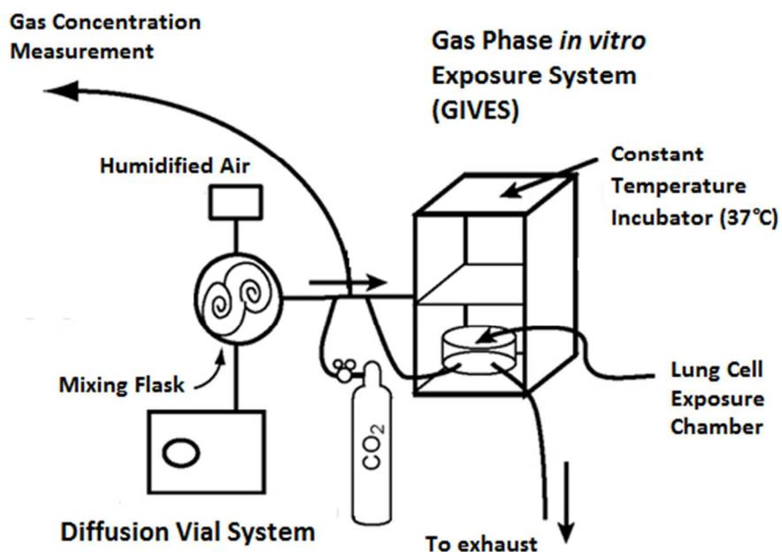
Schematic representation of the system design coupling a constant emission source from a diffusion vial to a gas phase *in vitro* exposure system (GIVES) for a direct air-liquid interface exposure to volatile organic compounds
