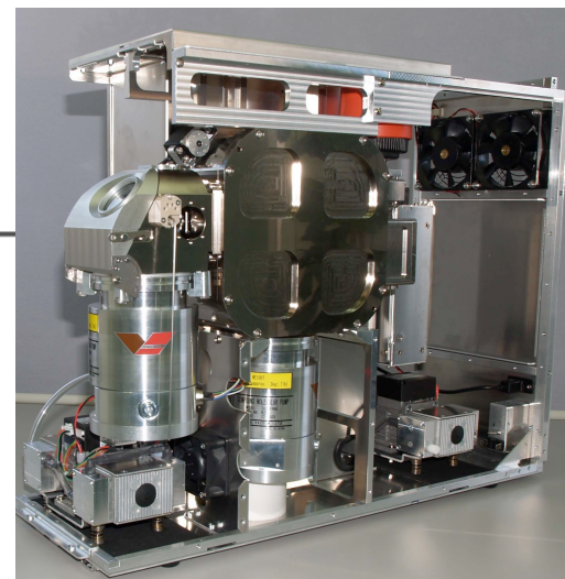
Miniaturized high-resolution TOF mass spectrometer "MULTUM-S II"
