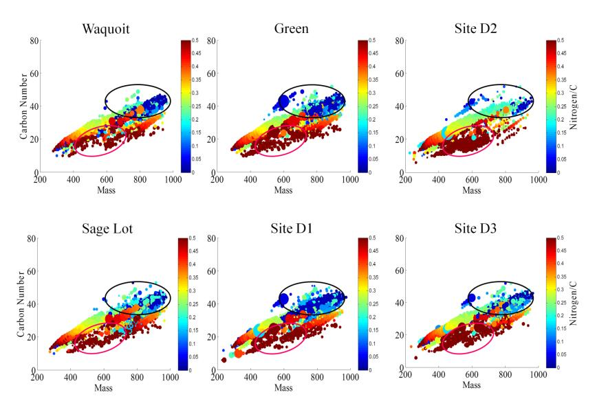
**Figure 2.** Carbon versus mass plots for the nitrogen containing features detected via ESI-FT-ICR-MS in the groundwater samples. Larger diameter denotes greater intensity and color indicates the N:C ratio. The pink oval marks the region of the plot that is
