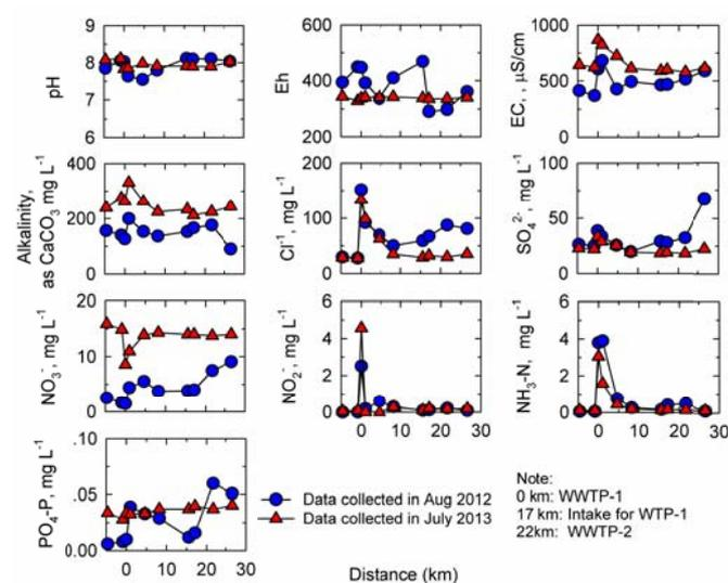
Figure 2. Concentrations of pH, Eh, alkalinity, EC,  $\text{Cl}^-$ ,  $\text{NO}_3^-$ ,  $\text{NO}_2^-$ ,  $\text{NH}_3\text{-N}$ ,  $\text{SO}_4^{2-}$ , and  $\text{PO}_4\text{-P}$  as a function of sampling distance.
