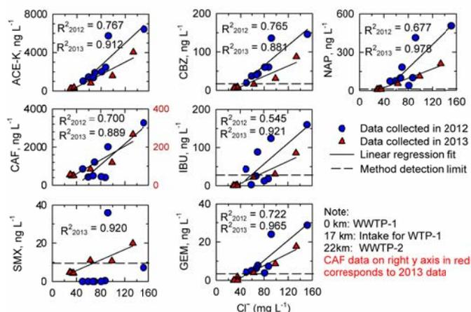
Figure 4. Concentrations of acesulfame-K (ACE-K), caffeine (CAF), sulfamethoxazole (SMX), carbamazepine (CBZ), ibuprofen (IBU), gemfibrozil (GEM), and naproxen (NAP) as a function of  $\text{Cl}^-$  concentration. The method detection limits of ACE-K and CAF were too low to appear in the figure.
