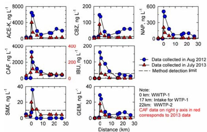
Figure 3. Concentrations of acesulfame-K (ACE-K), caffeine (CAF), sulfamethoxazole (SMX), carbamazepine (CBZ), ibuprofen (IBU), gemfibrozil (GEM), and naproxen (NAP) as a function of sampling distance. The method detection limits of ACE-K and CAF were too low to appear in the figure.
