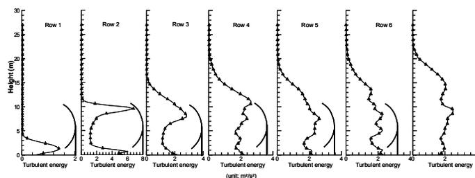
Fig. 6 Mean Velocity and Turbulent Energy Profiles Within parabolic trough collector Field
