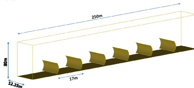
Fig. 4 The studied parabolic trough collector Field
