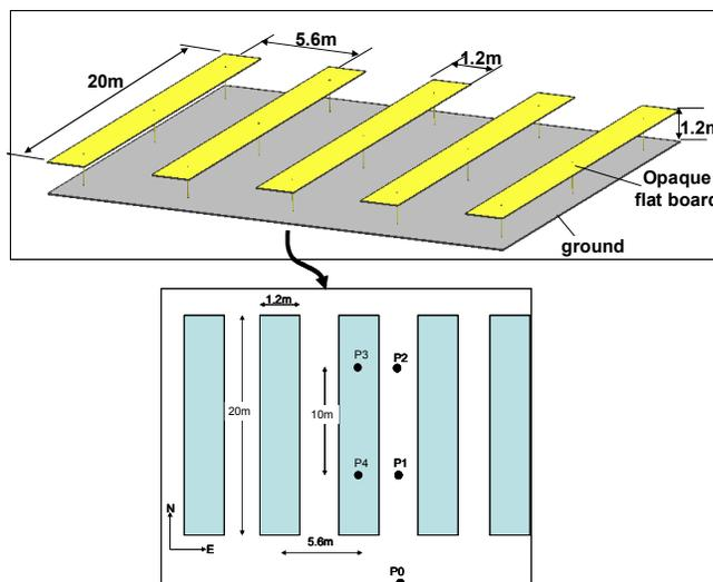
Fig. 9 General map of the experimental device. The top frame is the perspective view; the bottom frame is the planform.
