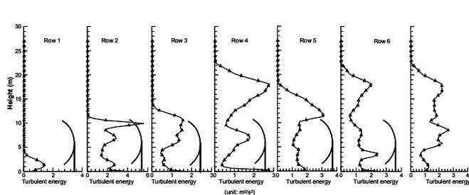
Fig. 5 Instantaneous Velocity and Turbulent Profiles Within parabolic trough collector Field
