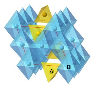
Fig. 1. The spinel crystal structure where the 'A' atoms occupy the tetrahedral sites, and the 'B' atoms occupy the octahedral site. Throughout this paper, the 'A' atoms are multivalent intercalating ions selected from the set  $\{Mg^{2+}, Ca^{2+}, Zn^{2+}, Y^{3+}, Al^{+3}\}$ , and the 'B' atoms are transition redox-active ions, selected from the set  $\{Ti, V, Cr, Mn, Fe, Co, Ni\}$ .
