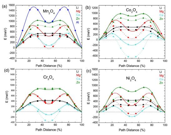
Fig. 7 Computed minimum energy paths for migration of different intercalants between the tetrahedral sites in the spinel  $B_2O_4$  (B = Mn, Co, Ni, Cr) at the high vacancy limit (solid line) and dilute vacancy limit (dotted line), i.e. one mobile specie per supercell (2x2x1 of primitive cell).
