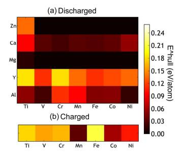
Fig. 5 a) The calculated thermodynamic stability of the  $AB_2O_4$  spinel compounds as a function of the intercalating ion (vertical axis) and redox metal (horizontal axis). (b) The energy above hull of the charged state which is calculated as the formation energy difference between a compound and the convex hull (see electronic supplemental information (ESI) for a detailed explanation).
