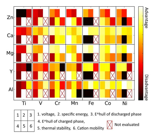
Fig. 8 Qualitative summary of multivalent spinel compounds based on multiple performance metrics, such as voltage, specific energy, thermodynamic stability of charged and discharged phases, thermal stability and intercalant mobility. The favorable (unfavorable) properties are represented with light (dark) color.
