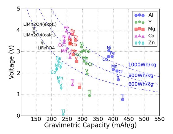
Fig. 2. The computed average voltage vs. gravimetric capacity for intercalation of A = Zn, Ca, Mg, Y and Al in various  $M_2O_4$  spinels up to composition  $AM_2O_4$ . The redoxactive metal is marked next to each point. Dashed curves show the specific energy of 600Wh/kg, 800Wh/kg and 1000Wh/kg, respectively. The spinel  $LiMn_2O_4$  and olivine  $LiFePO_4$  data points are also marked on the plot for comparison<sup>22,36,43</sup>.
