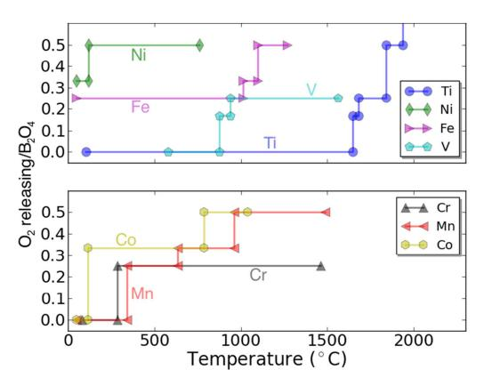
Fig 6. The calculated thermodynamic  $O_2$  evolution diagram of charged host spinel compounds as a function of temperature. The vertical axis denotes how much  $O_2$  is predicted to be released from the compound per formula unit of  $B_2O_4$  as the material decomposes.
