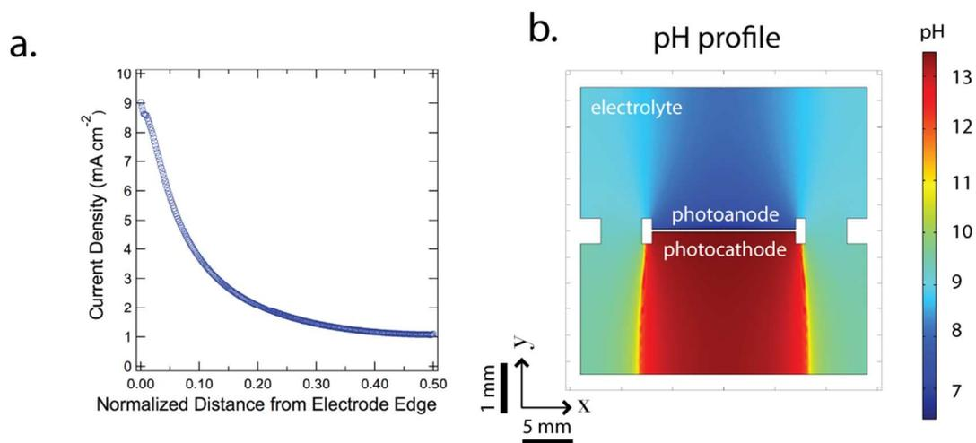
**Figure 3.** (a) Current density as a function of the normalized distance from the photoelectrode edge from the simulation, (b) Cross-sectional pH profiles in the membrane-free device from the COMSOL Multiphysics simulation.
