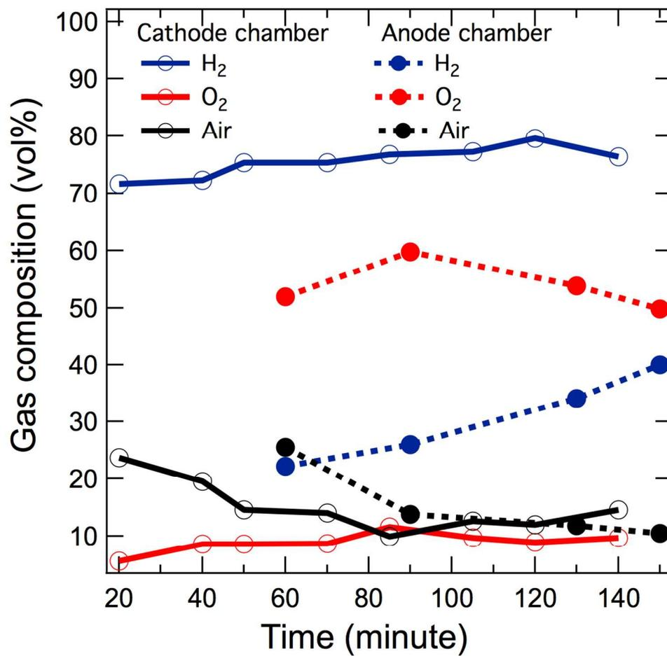
**Figure 4.** Time evolution of the gas composition (H<sub>2</sub>, O<sub>2</sub> and air) from the cathode compartment (solid lines) and the anode compartment (dashed lines).
