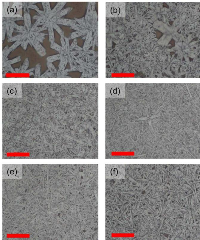
**Fig 1:** Optical microscopy images of spray-deposited thin-films of methylamine iodide and lead chloride onto substrates held at a range of elevated temperatures. (a) 28 °C, (b) 38 °C, (c) 55 °C, d) 75 °C, e) 80 °C, f) 87 °C. The scale bar in each image corresponds to 20 µm.
