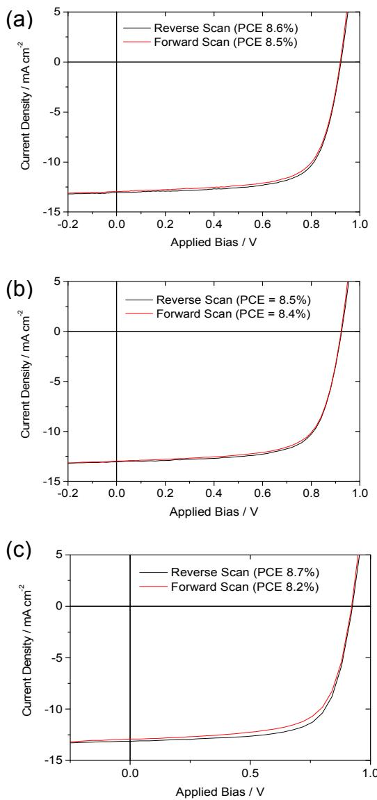
**Fig 4:** Current-density versus voltage characteristics for a perovskite solar cell device measured under different scan rates and scan directions: (a)  $0.5 \text{ V s}^{-1}$ , (b)  $1 \text{ V s}^{-1}$  and (c)  $2 \text{ V s}^{-1}$ . Efficiency values are shown in each figure legend. Note that the forward bias sweep conditions reported in part (b) correspond to our standard testing protocol.
