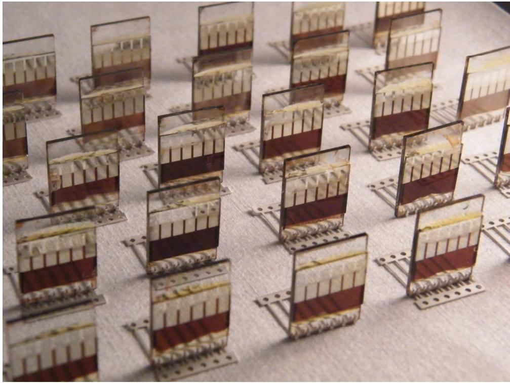
Perovskite solar cells prepared via spray-deposition of the active layer have been realized, advancing this promising technology towards roll-to-roll compatible processing methods.
