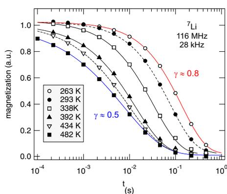
FIG. 10: Temperature-variable  ${}^7\text{Li}$  NMR  $R_{1\rho}$  transients recorded in the lab-frame using a spin-locking frequency of 28 kHz. Solid and dashed lines show fits with stretched exponentials. The stretching exponents  $\gamma_Q$  are shown as a function of  $T$  in Fig. 10.
