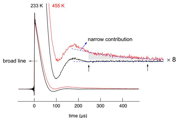
FIG. 9:  ${}^7\text{Li}$  NMR (transversal) transients of nanocrystalline  $\text{Li}_2\text{O}_2$  recorded with the spin-lock technique at 28 kHz and a Larmor frequency of 116 MHz. In contrast to the signal recorded at 233 K, the FID obtained at elevated  $T$  reveals a slowly decaying intensity which is responsible for the motionally narrowed NMR line visible in the Fourier transforms in Fig. 7.
