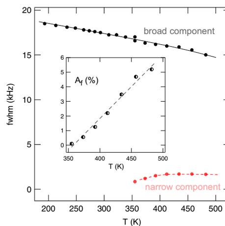
FIG. 8: Line widths (fwhm, full width at half maximum) of the two NMR components visible in the  ${}^7\text{Li}$  NMR spectra shown in Fig. 7.  $A_f$  denotes the area fraction, which also equals the *number fraction*, of fast diffusing Li spins in nanocrystalline lithium peroxide prepared by high-energy ball milling.
