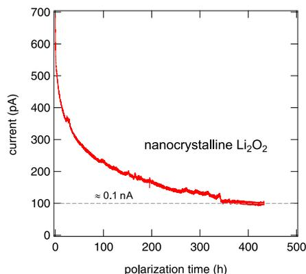
FIG. 6: Polarization curve (dc) of a nanocrystalline lithium peroxide prepared by high-energy ball milling. The electric contact to the pellet pressed was realized by plasma gold sputtering. The voltage applied across the pellet was 0.5 V. The almost constant current which is reached at long polarization time, that is the (quasi) stationary state, is slightly below 100 pA.
