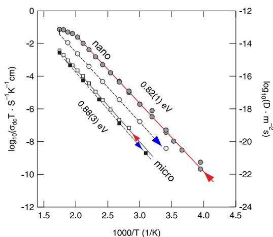
FIG. 5: Arrhenius plot of the total conductivity of nanocrystalline and microcrystalline  $\text{Li}_2\text{O}_2$  when measured in a flow of dry nitrogen. The arrows denote the heating and cooling runs, respectively. The activation energies refer to the heating runs. During cooling we obtain 0.90(7) eV (micro) and 0.83(7) eV (nano). To obtain the right axis  $\sigma_{dc}$  values have been roughly converted into solid-state diffusion coefficients  $D$  via the Nernst-Einstein equation.
