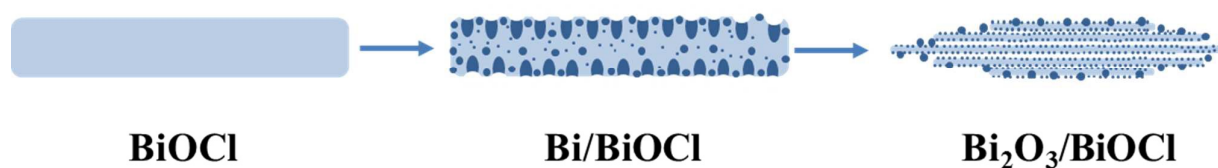
Fig.5 Schematic diagram of the hierarchical structure and forming process of \text{Bi}_2\text{O}_3/\text{BiOCl} heterojunctions
