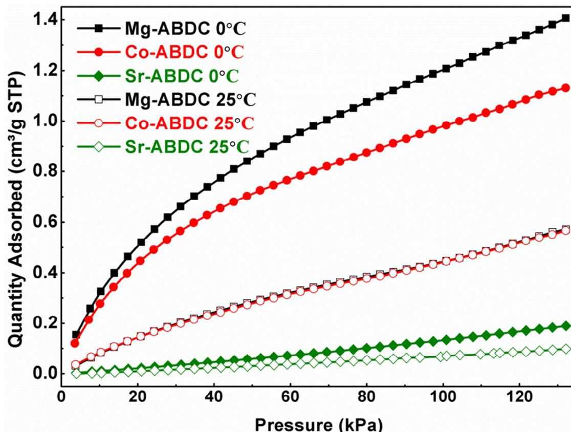
**Fig. 6** CO<sub>2</sub> adsorption at 0 °C and 25 °C on M-ABDC (M = Mg, Co, Sr).
