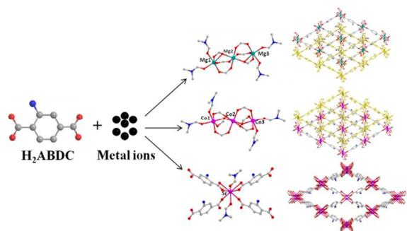
Three new amino-functionalized MOFs based on 2-aminoterephthalic acid with Mg(II), Co(II) and Sr(II) ions.
