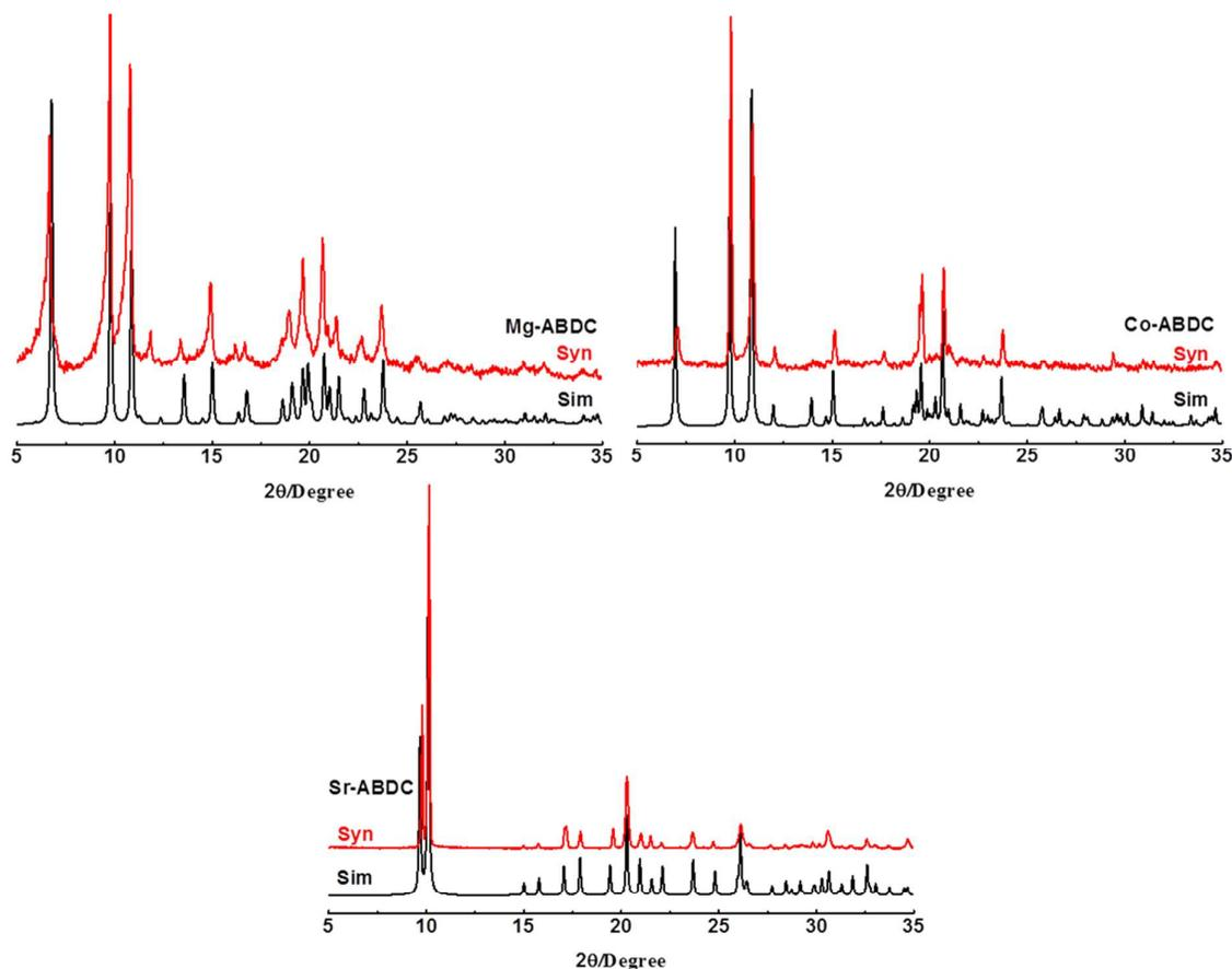
**Fig. 3** Comparison of XRD patterns from synthesis (red) and simulation (black).
