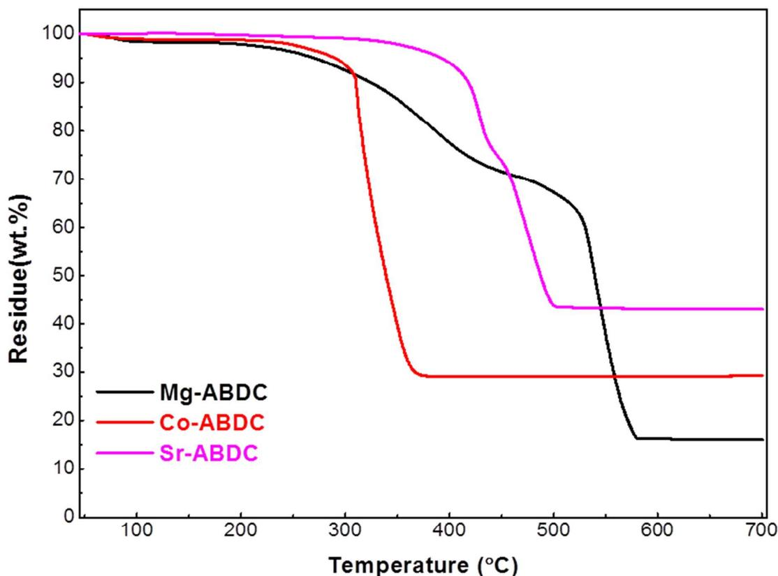
**Fig. 4** Weight loss (TGA) curves of Mg-ABDC, Co-ABDC and Sr-ABDC measured in air at a heating rate of 5 °C/min
