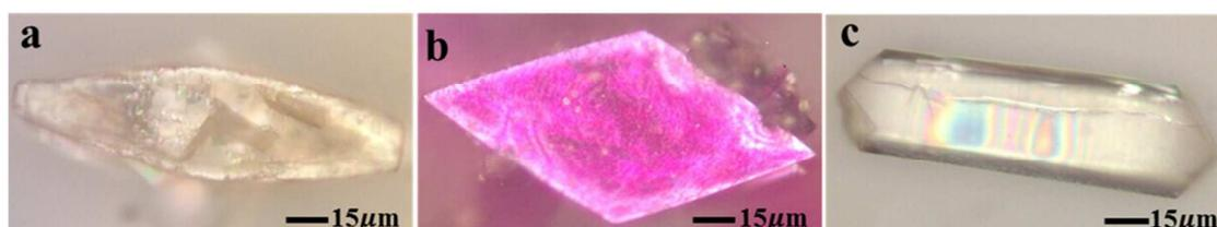
**Fig. 2** Optical images at 200x magnification of (a) Mg-ABDC, (b) Co-ABDC and (c) Sr-ABDC.
