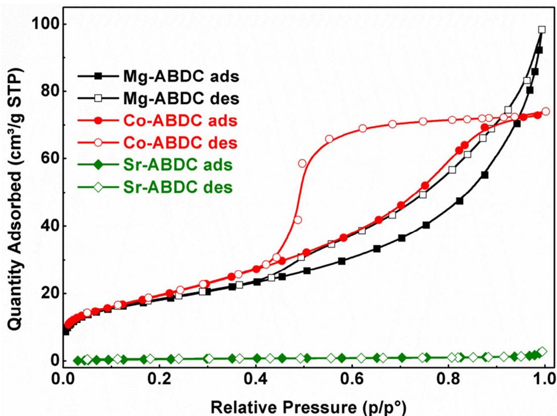
Fig. 5 N<sub>2</sub> ads-desorption isotherms measured at -196 °C.
