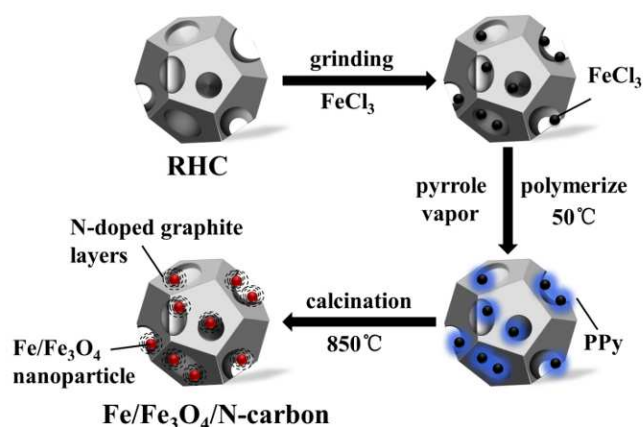
Scheme 1 Schematic illustration of the formation of the Fe/Fe 3 O 4 /N-carbon composite.
