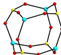
**Figure 12:** Core structure of **6** resembling a D4R cubane structure.
