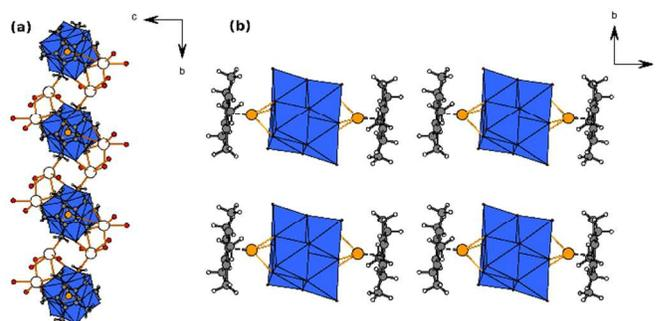
**Fig. 2.** (a) Crystal packing of **1** showing the connectivity between  $\text{K}^+$  cations (white) and the Lindqvist entity; (b)  $\pi$ - $\pi$  interactions between the aromatic  $\text{C}_5$  rings of two adjacent Lindqvist entities in **1**.
