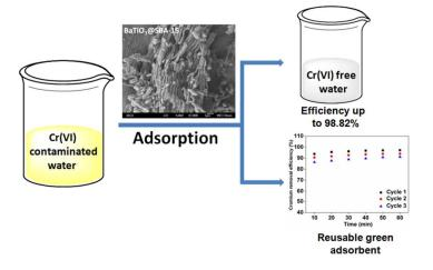
BaTiO<sub>3</sub>@SBA-15 nanocomposite material has been synthesized via solid state reaction route and it is successfully employed as an adsorbent for the removal of chromium(VI) from contaminated water with very high adsorption efficiency and only 40 min contact time in a batch reactor.
