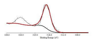
Fig. 3 V2p high-revolution XPS spectrum of the as-synthesized sample.
