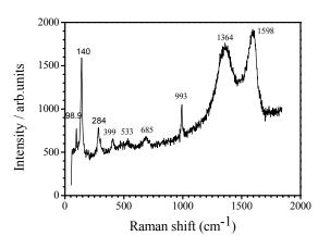
Fig. 5 Raman spectrum of graphene based composite.
