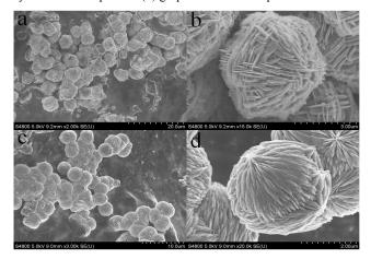
**Fig. 2** SEM images of the as-synthesized materials (a, b) and <sup>30</sup> graphene based composite (c, d).
