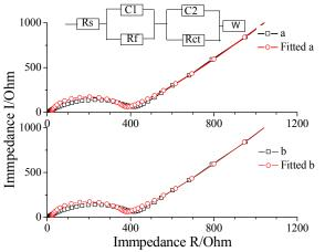
**Fig. 8** Nyquist-diagram of graphene based composite (a) and  ${}^{5}$  VO<sub>2</sub>•1.65H<sub>2</sub>O (b) after discharging and charging for 1 cycle (inset is the fitting impedance circuit model).
