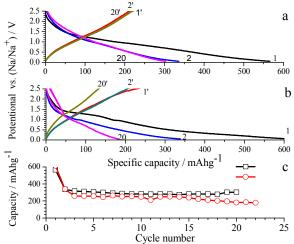
**Fig. 7** The 1<sup>st</sup>, 2<sup>nd</sup> and 20<sup>th</sup> charge-discharge profiles of (a) graphene based composite, (b) VO<sub>2</sub>•1.65H<sub>2</sub>O semi-microspheres and (c) The cycling performance of vanadium oxide hydrate <sup>35</sup> semi-microspheres (○) and graphene based composite (□).
