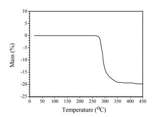
35 Fig. 4 TG curve of the as-synthesized sample.
