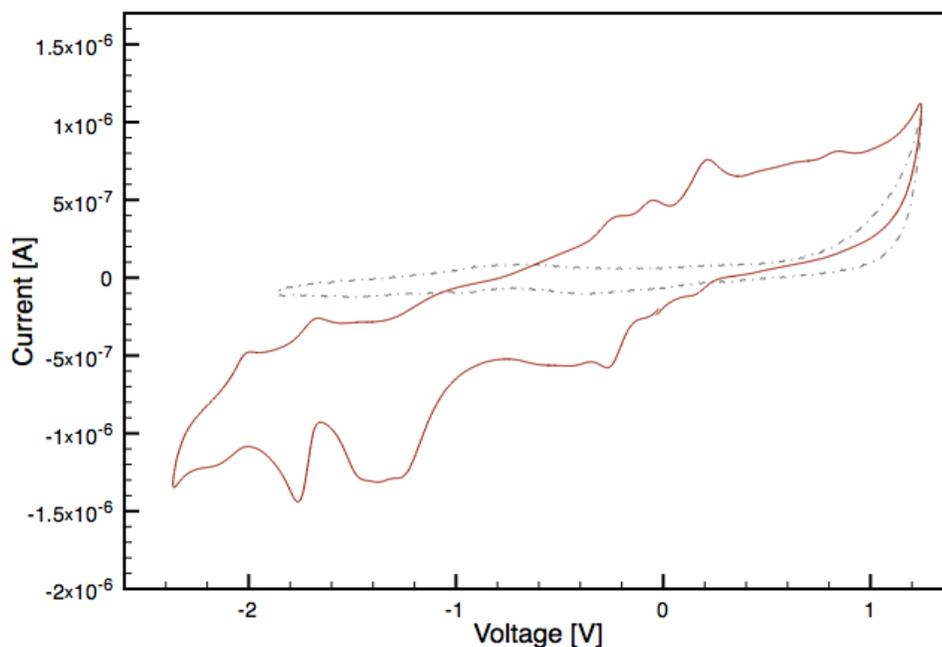
**Fig. 7** Cyclic voltammograms, 0.001 M  $[\text{Fe}(\text{vox})_3]$  in DMSO (red), 0.1 M tetra(*n*-butyl)ammonium perchlorate, scan rate  $100 \text{ mV} \cdot \text{s}^{-1}$  (background, grey).
