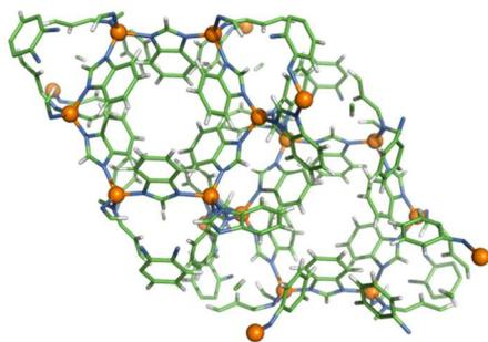
**Figure 1.** The unit cell of ZIF-7 and ZIF-9. Zn/Co: orange, C: green, N: blue, H: silver.
