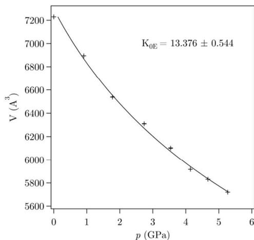
**Figure 4.** The evolution of the unit cell volume of ZIF-9 as a function of hydrostatic pressure, completed with EoS fit.
