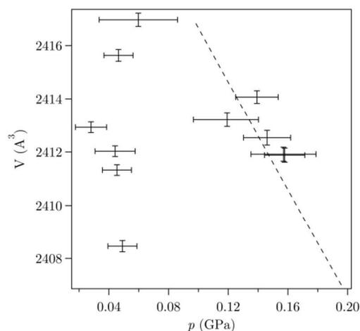
**Figure 3.** Pressure-induced oversaturation reflected by an increase in volume upon pressurisation at low pressure. Dashed line is the EoS fit at higher pressure.
