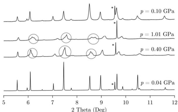
**Figure 2.** X-ray diffraction peak splitting upon increasing pressure and recovery at low pressure in Experiment A. The diffraction peak from quartz standard is indicated by \*.
