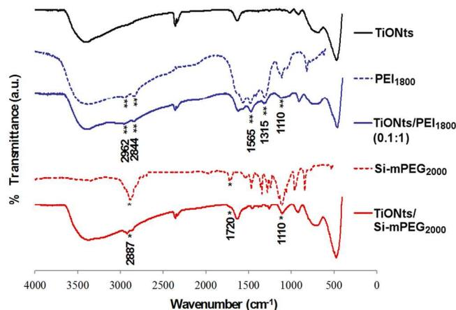
Fig. 6 FTIR spectra of bare TiONts, PEI<sub>1800</sub>, TiONts/PEI<sub>1800</sub> (1:1, w:w) nanohybrid, Si-mPEG<sub>2000</sub> and TiONts/Si-mPEG<sub>2000</sub> nanohybrids.
