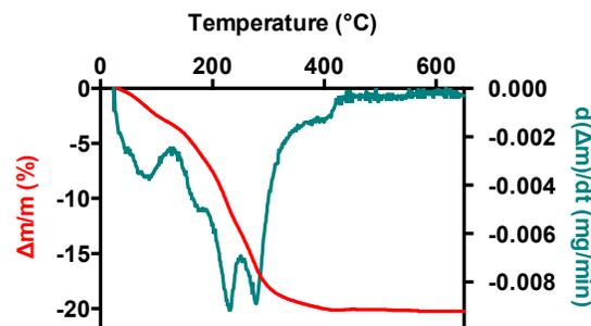
**Fig. 2** TGA with derivative weight of TiONts/PEG<sub>2000</sub> from room temperature to 650 °C.
