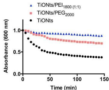
Fig. 5 Stability of TiONts, TiONts/PEG<sub>2000</sub> and TiONts/PEI<sub>1800</sub> suspensions over 150 min following their absorbance at 600 nm and pH = 7.
