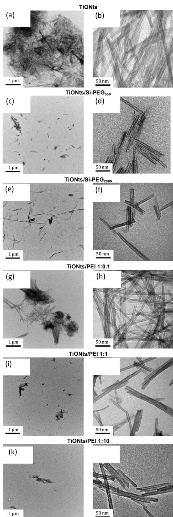
**Fig. 3** TEM images of (a-b) bare TiONts, (c-d) TiONts/Si-PEG<sub>550</sub>, (e-f) TiONts/Si-PEG<sub>2000</sub>, TiONts/PEI<sub>1800</sub>: (g-h) 1:0.1, w:w, (i-j) 1:1, w:w, (k-l) 1:10, w:w.
