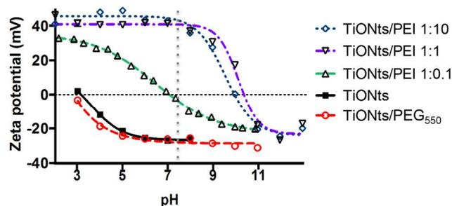
**Fig. 4** Zeta potential versus pH of bare TiONts, TiONts/PEI<sub>1800</sub> and TiONts/PEG<sub>550</sub> nanohybrids as a function of pH (in NaCl 10<sup>-2</sup> mol.L<sup>-1</sup>).
