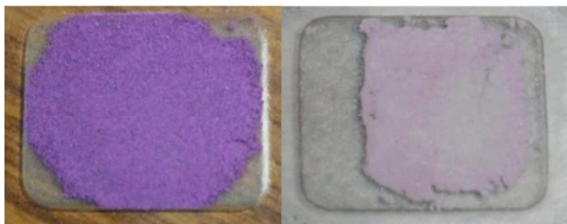
Fig. 1. Colors of Na 2 Co[PO 4 ]F samples prepared under atmospheric pressure (left), and 3 GPa (right).
