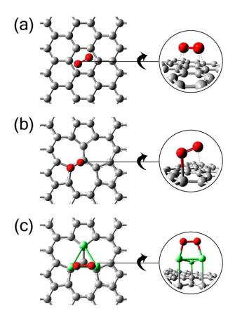
Fig. 6: Optimized configurations for dioxygen adsorption: (a)  $O_2$  - Pristine Graphene (b)  $O_2$  - DV(555-777) (configuration: A<sub>757</sub>-A<sub>777</sub>; (above B<sub>77</sub>)) (c)  $O_2$  - 3A<sub>757</sub>
