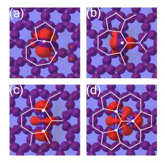
Fig. 5: Top view of deformation charge density isosurfaces (isovalues: 0.01 e/ Å<sup>3</sup> (red) and -0.01 e/ Å<sup>3</sup> (blue)) for (a)  $B_{75}$ , (b) T, (c)  $2A_{757}$  and (d)  $3A_{757}$  configurations.
