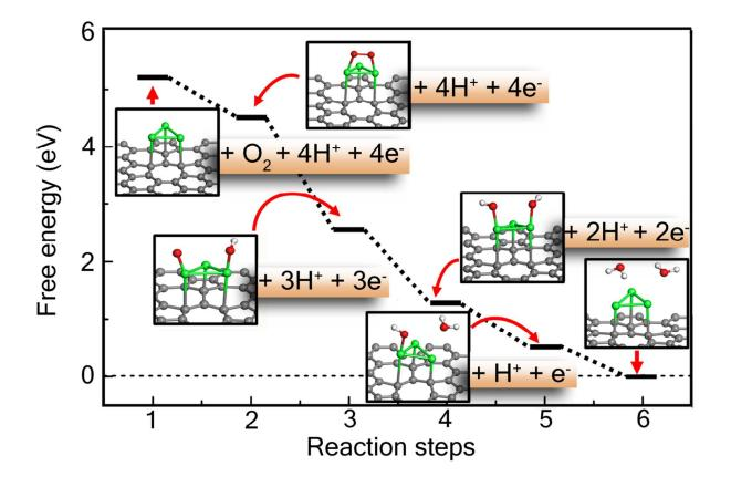
Fig. 7: Changes of free energy during oxygen reduction reaction while using As decorated DV(555-777) defect graphene as electrocatalyst. Optimized structures of the reactants during intermediate steps are shown in insets.
