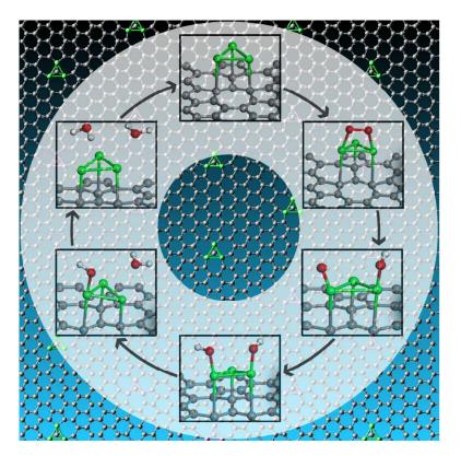
Arsenic adsorbed double vacancy defect graphene systems are found to demonstrate excellent electrocatalytic properties for oxygen reduction reaction via high affinity towards four electron process.
