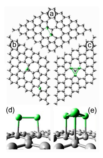
Fig. 3: Optimized structures of multiple As adatoms adsorption on DV(555-777) defect graphene system: (a)  $2A_{757}$ , (b) T-B<sub>66</sub>, (c)  $3A_{757}$ , (d) and (e) close up side views of  $2A_{757}$  and  $3A_{757}$  configurations respectively.
