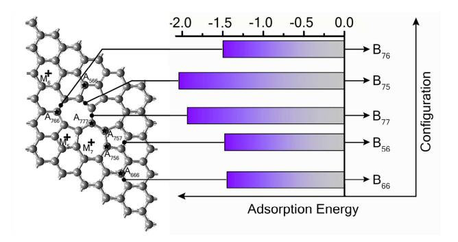
Fig. 1: Schematic representation of the most symmetric adsorption sites on DV(555-777) graphene system: A, B and M denote atop, bridge and middle sites (Exact positions of them are shown by star, dot and plus symbols respectively). The bar chart shows variation of single As adatom adsorption energies at different B sites.
