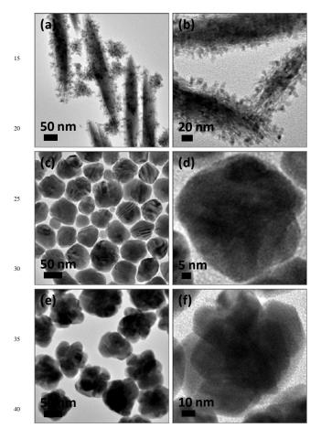
**Fig. 4** TEM images (a,c,e) and HRTEM images (b,d,f) of the HgS nanocrystals synthesized in OA/OLA mixture with volume ratio of 1/2 at 60°C (a,b), 100°C (c,d), and 150°C (e,f), respectively, by sulfidation of 45 Hg(II) ions with element sulfur.
