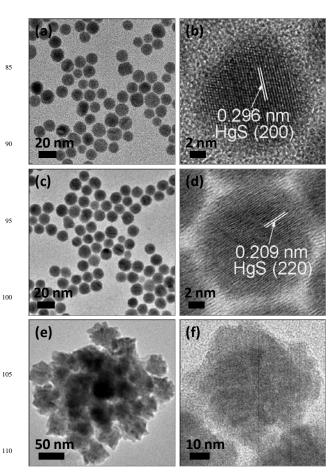
**Fig. 2** TEM images (a,c,e) and HRTEM images (b,d,f) of the HgS nanocrystals synthesized by sulfidation of Hg(II) ions with element sulfur in toluene (a,b) at room temperature, in oleylamine (c,d), and in oleic acid <sup>115</sup> (e,f) at elevated temperature.
