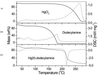
110 Fig. 1 TG-DSC curves of Hg(NO<sub>3</sub>)<sub>2</sub>, dodecylamine (DDA), and Hg(II)-DDA complexes formed by phase transfer technique.
