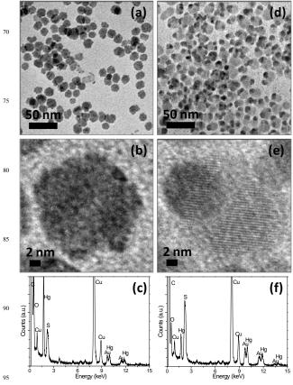
**Fig. 5** TEM images (a,d), HRTEM images (b,e), and EDX analyses (c,f) of the HgS-Au nanocomposites formed by mixing  $HAuCl_4$  and HgS nanocrystals in toluene for 8 h (a,b,c) and 12 h (d,e,f), respectively.
