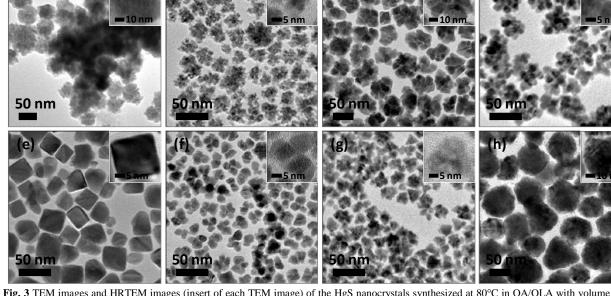
Fig. 3 TEM images and HRTEM images (insert of each TEM image) of the HgS nanocrystals synthesized at 80°C in OA/OLA with volume ratio of 1/0 (a), 1/1 (b), 1/2 (c), 1/3 (d), 1/5 (e), 2/3 (f), 2/1 (g), and 5/1 (h), respectively.
