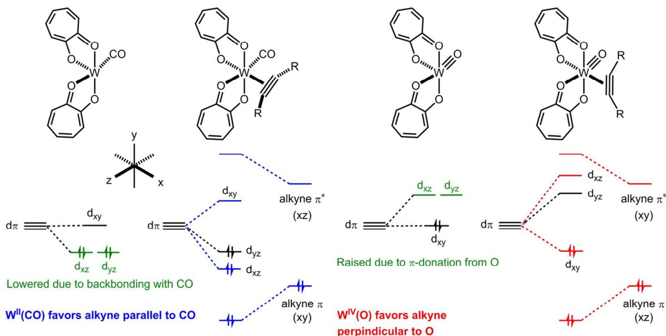
Figure 7. d-orbital splitting diagrams for  $W^{IV}$  oxo alkyne species.
