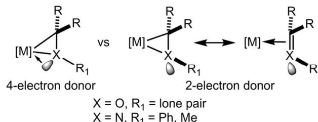
Figure 1. Coordination of ketones and imines as 2 and 4 electron donors.
